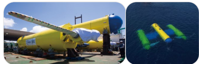
Figure 1.15 Field testing of Japan's first ocean current turbine in 2018
