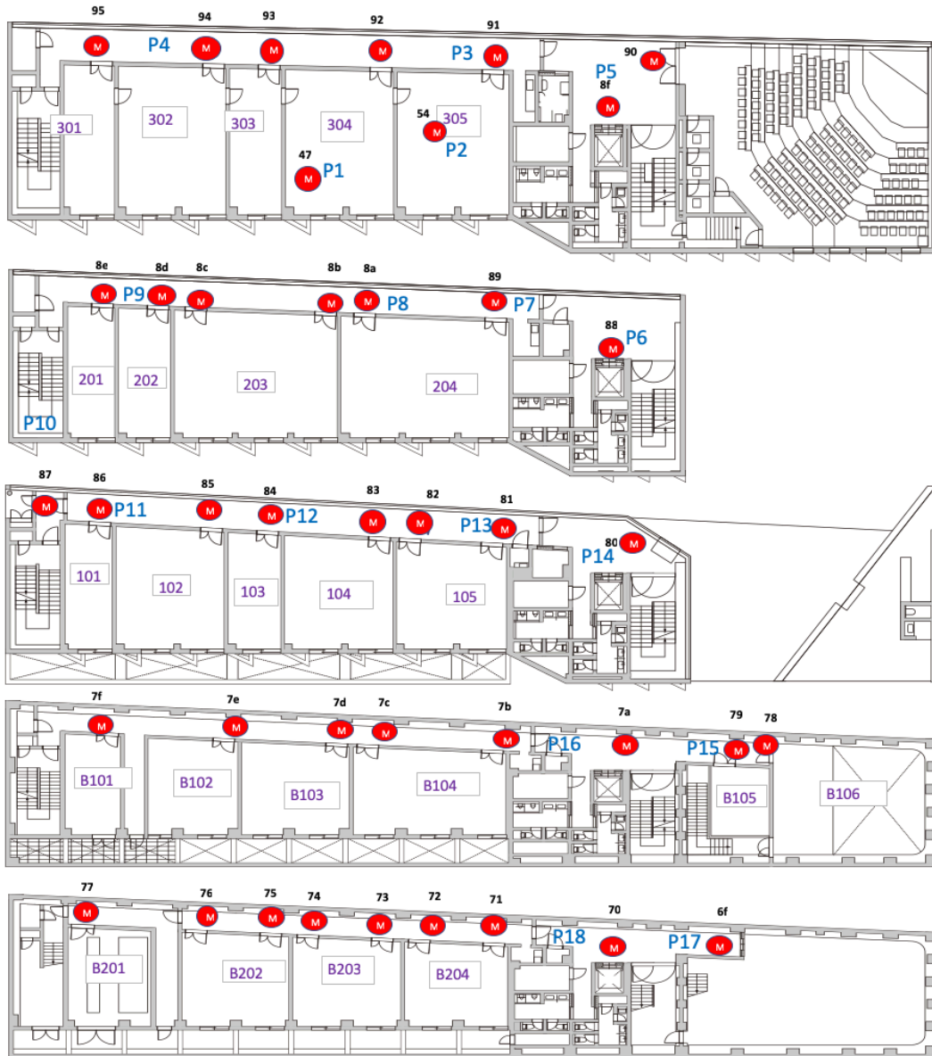
Figure 5.7: The deployment of BLE beacon inside the building
