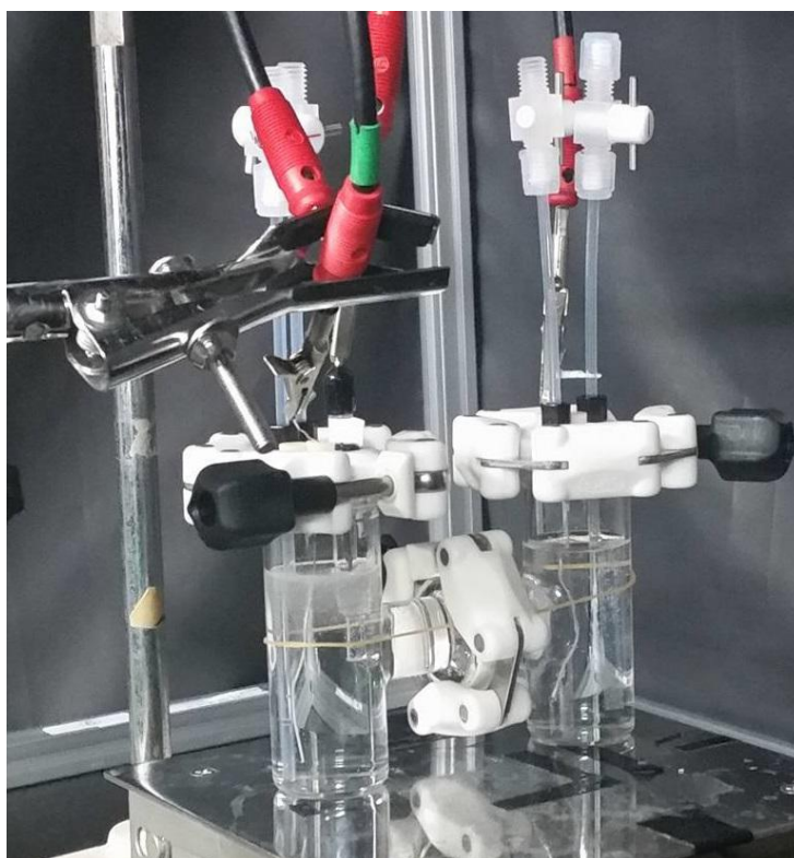
Fig. 3.2 Actual picture of the Electrochemical Cell
