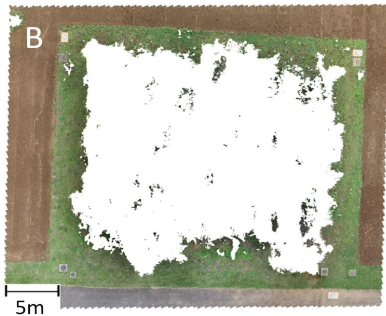
Fig. 3- 5 Results in the process to extract ground points from 3D dense point cloud. A: Cross section (the upper figure) in height of all dense point cloud including tree canopy and that (the lower figure) of the extracted ground level points in red belt in Fig. 3- 3B. B: 3D view from the top of dense point cloud at the extracted ground level.
