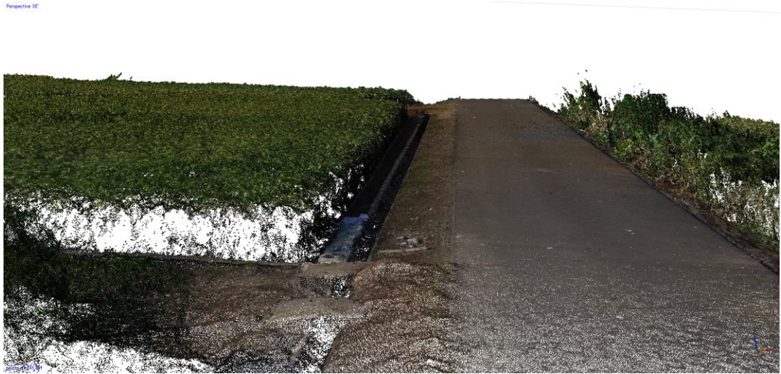
Fig. 2- 4 3D dense point cloud models reconstructed at sampling rate of 6 still images
