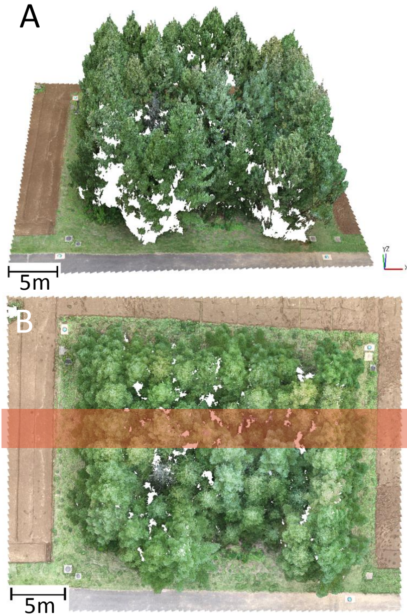
Fig. 3- 3 Examples of 3D dense cloud models reconstructed from a series of color images captured with the 28 mm lens. A: 3D model view from 40^\circ of depression. B: 3D view from the top. Red belt in Fig. 2B shows an area used to make the histogram in Fig. 3- 5.
