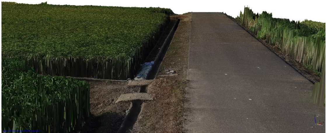
Fig. 2- 6 3D texture mapping models reconstructed at sampling rate of 6 still images /s.
