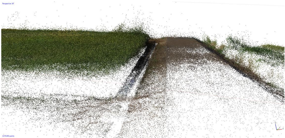
Fig. 2- 3 3D point cloud models reconstructed at sampling rate of 6 still images /s.
