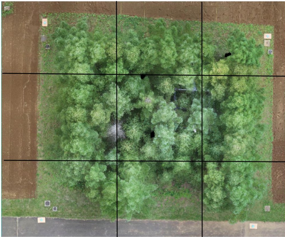
Fig. 3- 2 2D color image reconstructed from a series of color images captured with the 28 mm lens. The sections surrounded by black lines show nine divisions for DTM reconstruction.
