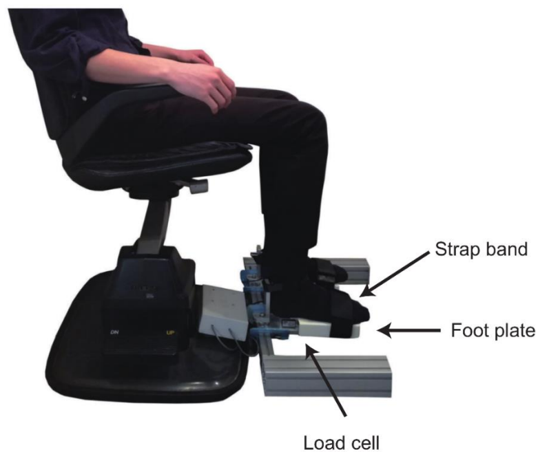
Figure 1. Experimental setup of the force match test. Participants were seated with hip and knee flexion and ankle dorsiflexion at 90^\circ . Each foot was strapped on to a separate metal foot plate, each constraining a load cell.
