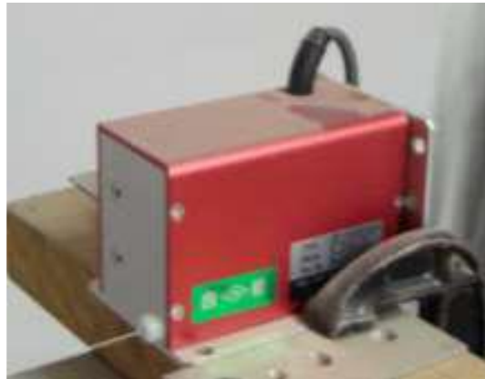
(a) External potentiometer instrument in Torsional Shear Apparatus
