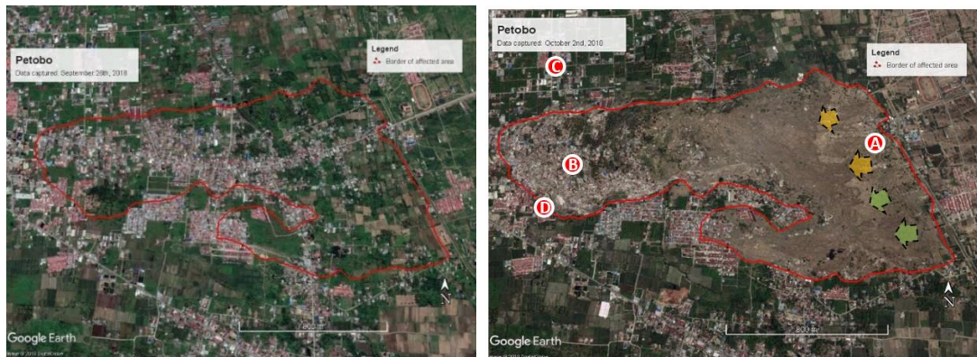
Figure 1-7 Condition before the earthquake (left) and the condition aftermath (right) (Hidayat, et al., 2020)
