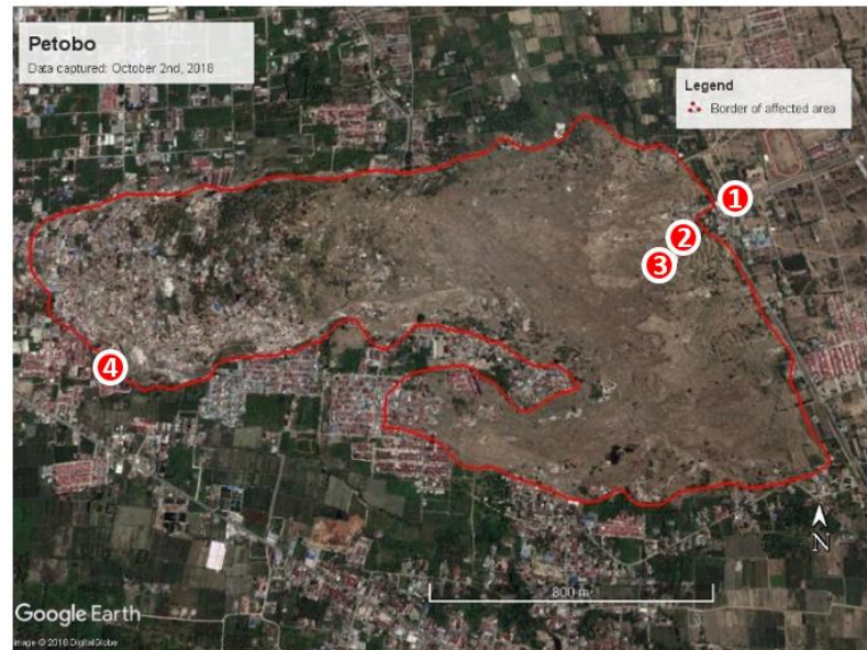
Figure 1-9 Location of DCPT test at Petobo, highlighted by the red circle. Points 1 and 4 are outside the affected areas while points 2 and 3 are near the crown area (Hidayat, et al., 2020).
