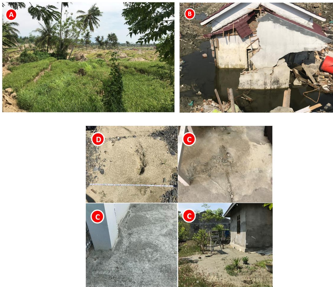
Figure 1-8 Tensile crack on soil body due to the earthquake motion (Point A), Inundation at the bottom part of the debris zone found at Petobo (Point B), and sand ejecta found in the non-affected area (Point C and D) (Hidayat, et al., 2020).
