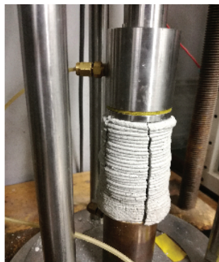
During the loading test linear cracks were observed
