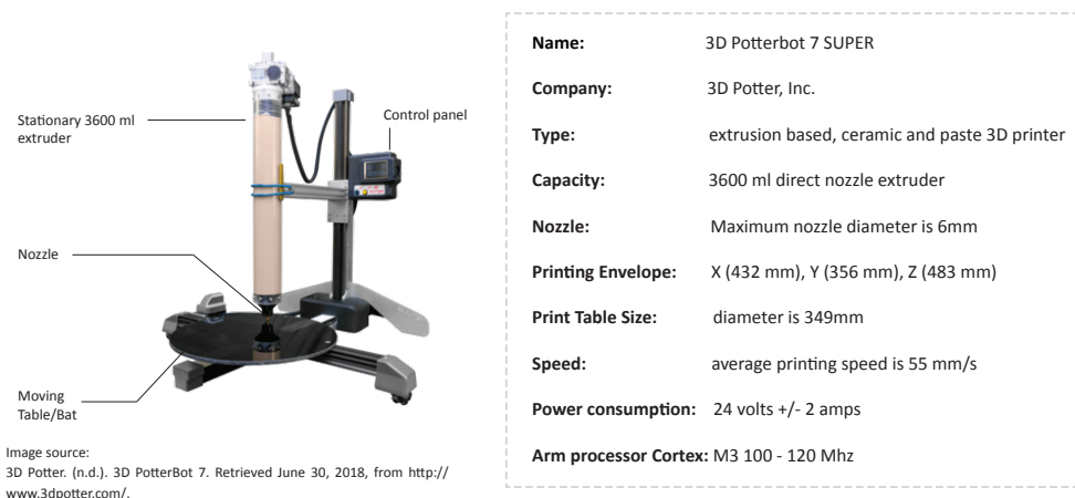
Figure 2.15. 3D Potterbot 7 SUPER Specifications
