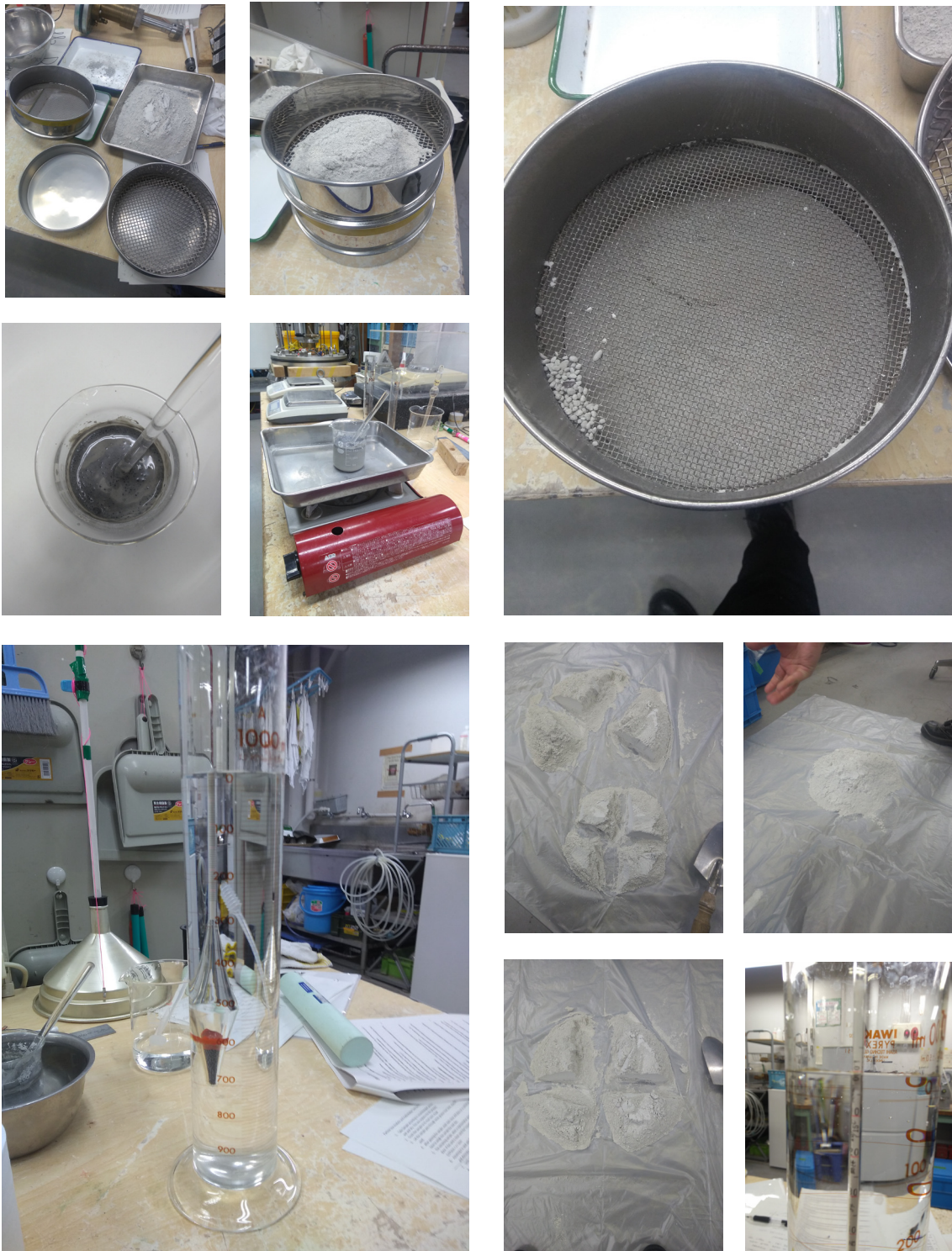
Figure 3.10. Test Method for Particle Size Distribution of Soils 'Dry Method' (JGS 0131- 2009)
