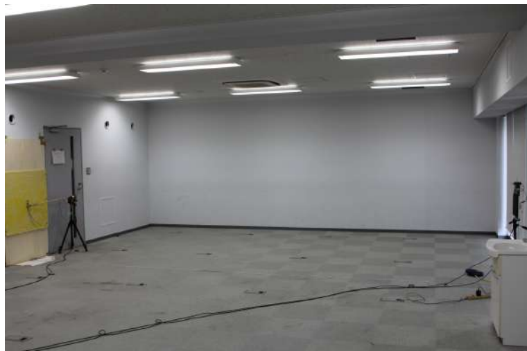
図 5.14: Arrangement to in-situ measurement of absorption properties at normal incidence
