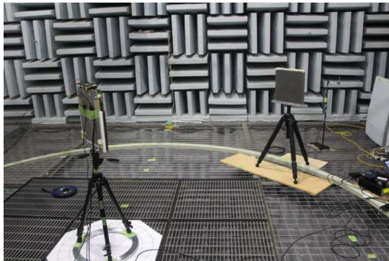
図 4.10: Geometrical setup in radiation directivity measurement
