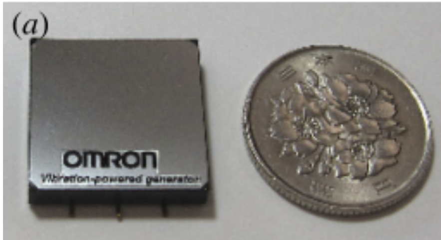
Figure 1-12 A fully-integrated linear-vibration electret energy harvester [45].
