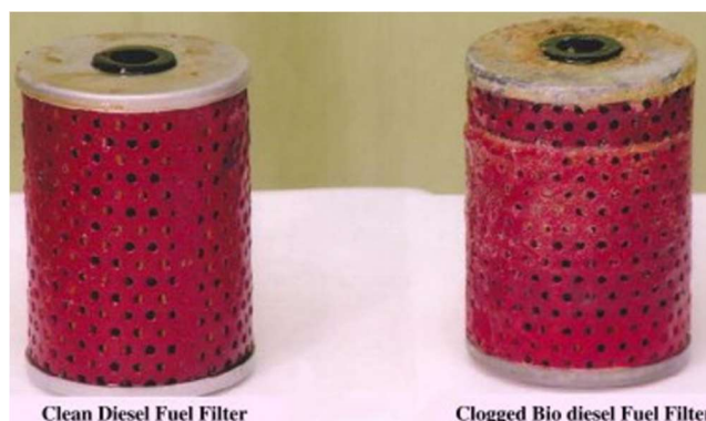
Fig. 1.1.3 Filter clogging problem with 100% biodiesel operated engine [5].
