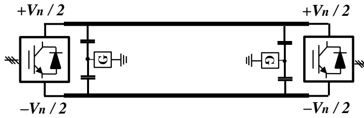
Fig. 1.6. Symmetric monopole configuration [5]
