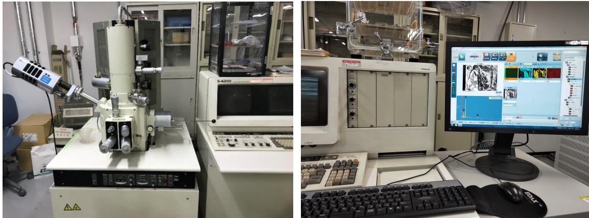
Fig. 2-5. SEM-EDS facility and computer operation window.
