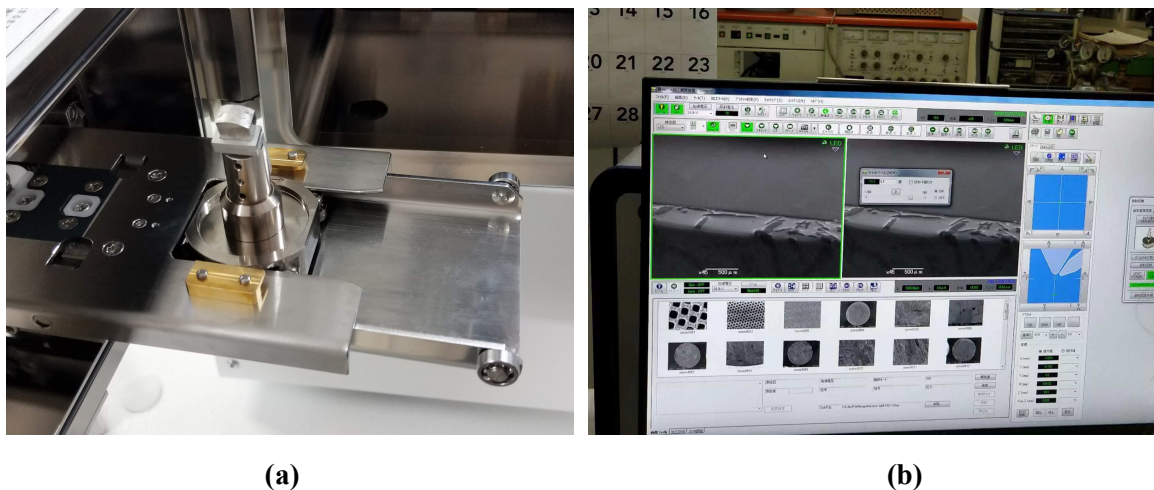
Fig. 2-7. (a) Sample on holder in EBSD chamber and (b) observation scene.
