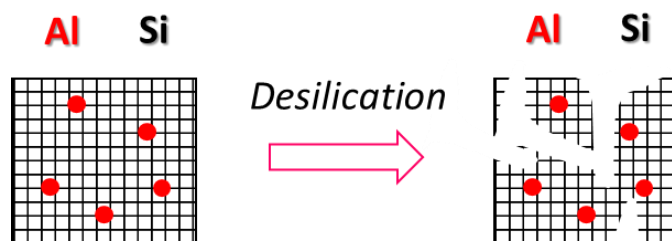
Figure 19. Schematic images of alkali leaching.
