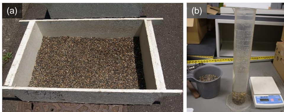
Fig. 2.5 (a) Sieving sediment particles and (b) estimating particle diameters.
