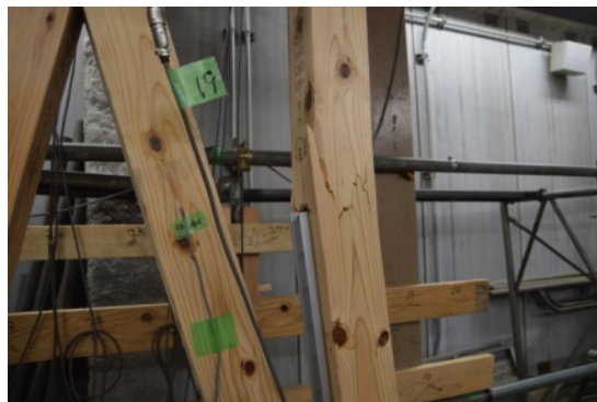
(c) 柱の引張り曲げ破壊 (NCLS-3)
