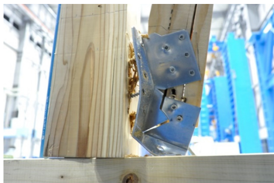
(a) 引張側筋かい金物の破断 (HS-1)
