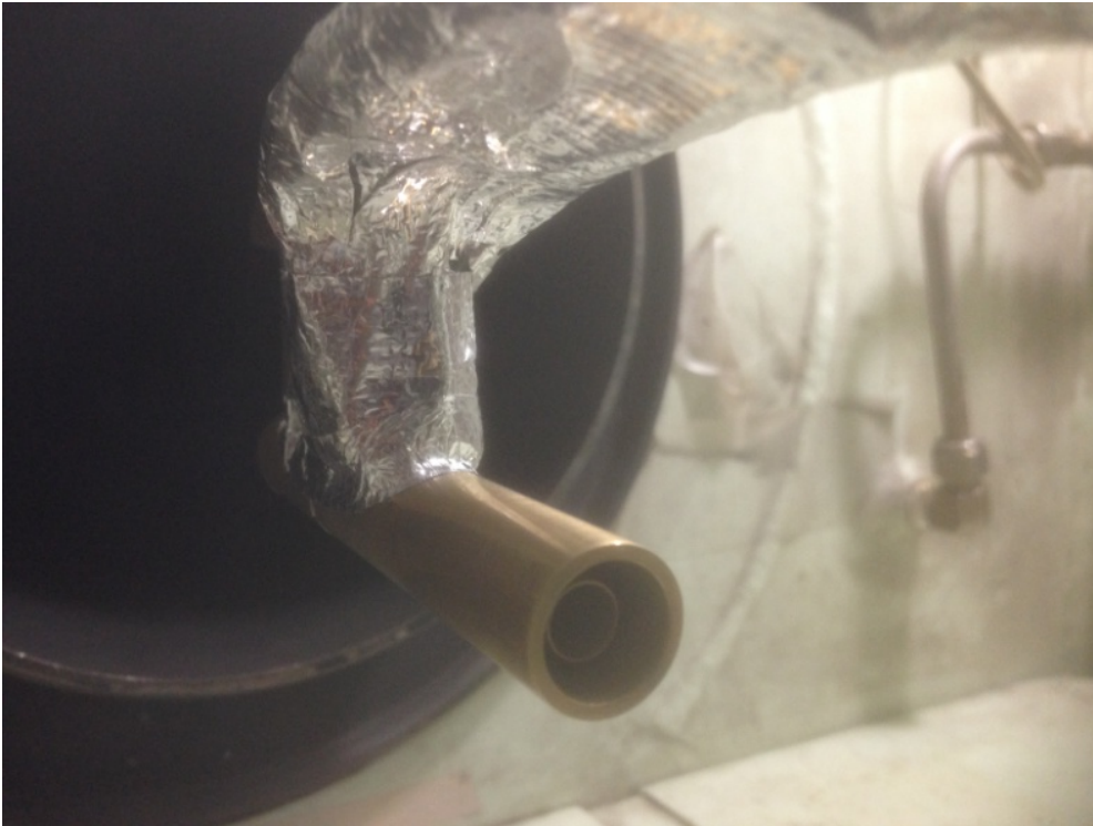
Figure 3.6 Experimental model Coaxial Jets Nozzle Back View
