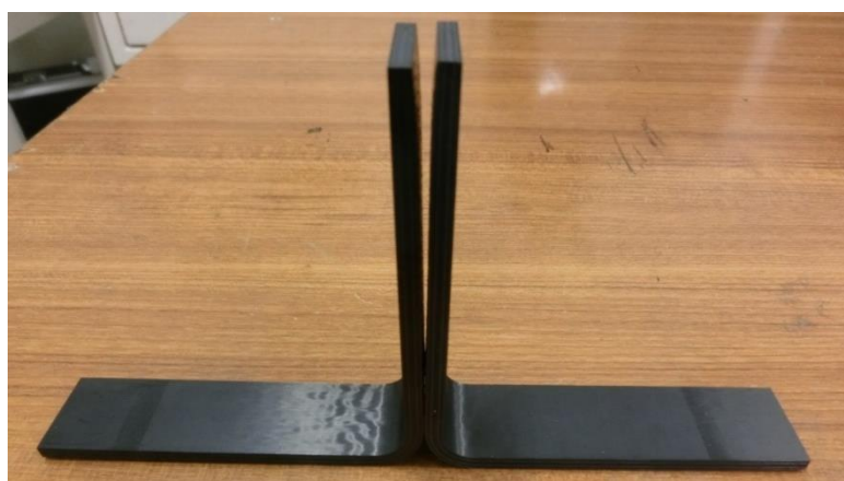
Fig. 1.10 Spring-in deformation in composite L-shaped parts.
