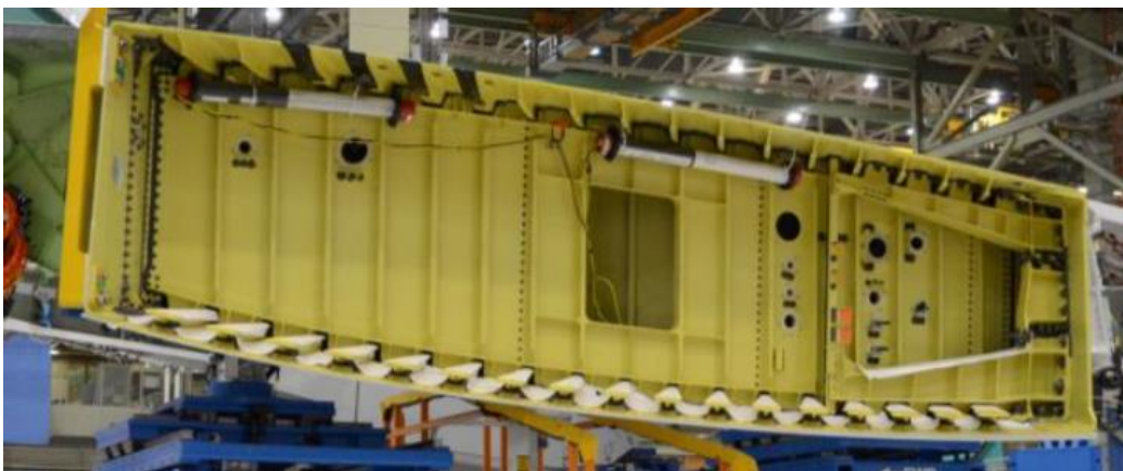
Fig. 1.13 Wing box root section of B787[15].
