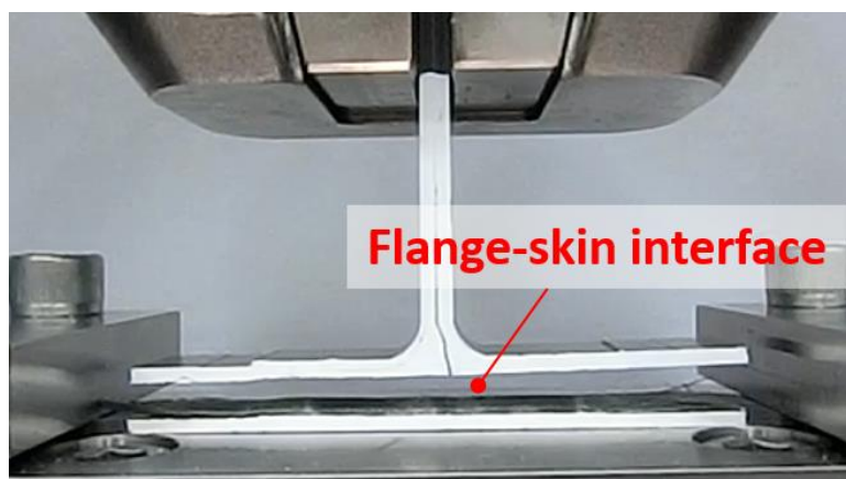
Fig. 1.14 Failure along flange-skin bonding interface.
