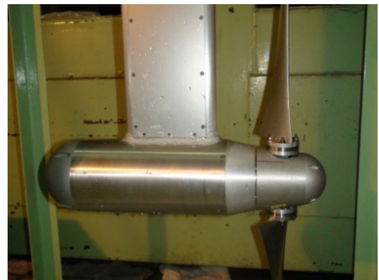
Fig 3 1/50 scale model of two bladed horizontal axis ocean current turbine
