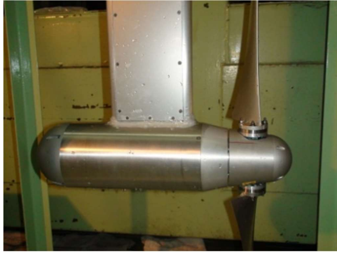
Fig A.10 1/50 scale model of two bladed horizontal axis ocean current turbine
