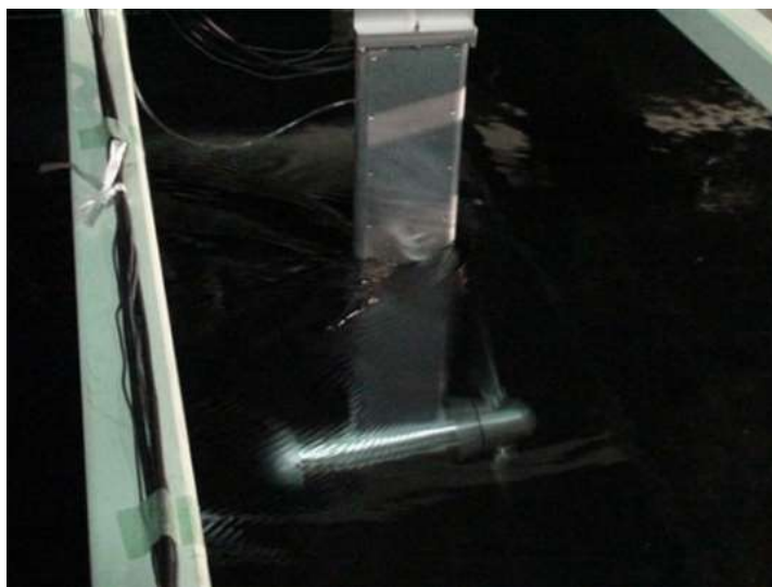
Fig A.12 Model turbine in the circulating water channel at 0.48 m/s
