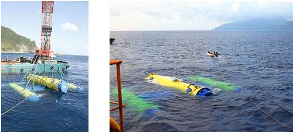
Fig 1.4 Verification test of the ocean current turbine off Kuchinoshima [34]
