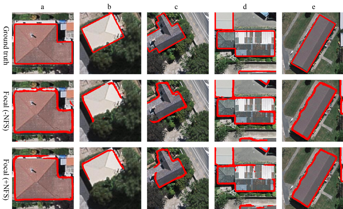
Figure 4.8: Representative results of outline extracted by focal loss that with/without nearest feature selector(NFS). The background and red line represent aerial input and outline, respectively.
