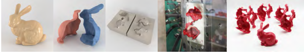
Figure 3.1: From left to right: We propose a method to decompose an input shape (surface mesh) into molding-ready shell pieces and to generate the corresponding 3D printable molds. Using, for example, an injection molding machine, we can fabricate many physical replica at low cost and in a short amount of time.
