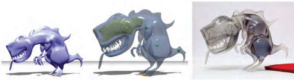
Figure 2.1: Make it stand [52] automatically optimizes gravitational properties of the input shape. This figure is adapted from the Figure 1 of [52].
