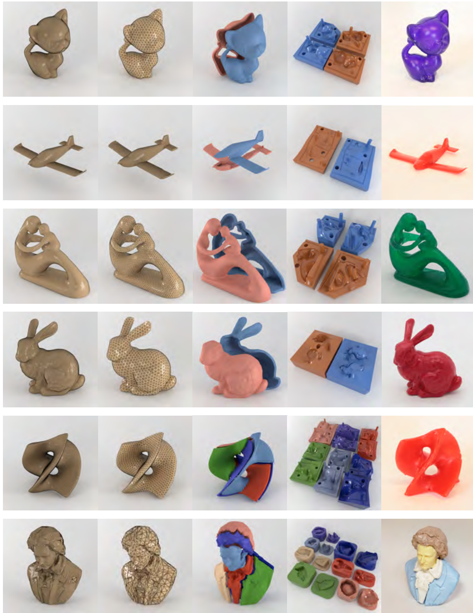
Figure 3.18: (From left to right) High-res detailed input \mathcal{S}_{\text{input}} , low-res representation \mathcal{S}_{\text{low}} , final decomposition, corresponding automatically generated mold pieces, and fabrication results. (From top to bottom) We denote our examples as kitten, airplane, fertility, bunny, sculpture, and Beethoven. Each pair of mold pieces corresponding to the part with the same color. Bunny example is designed for injection molding, and the others are designed for manual resin casting. For the Beethoven model, we omit the computation of the smooth surface during the mold generation.
