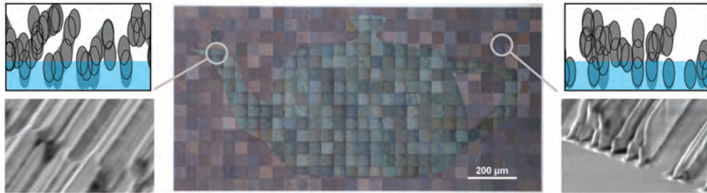
Figure 2.4: Printed object with structure color by using [5]. A silhouette of a teapot is colored in blue, and the background is colored in red. Both color are structure color and no color pigment is used. This figure is adapted from the Figure 1 of [5].
