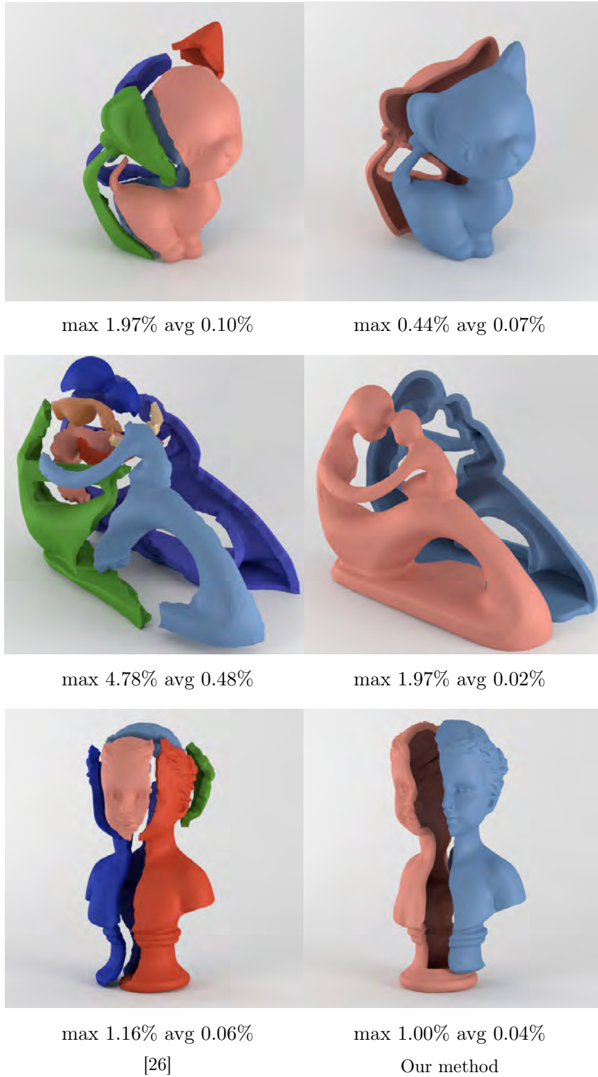
Figure 3.17: Side-by-side comparison of [26] and our method. From top to bottom: Kitten, fertility, and bust sculpture. The average and maximal Hausdorff distances to the input mesh are given as ratio with respect to the model’s bounding box diagonal.
