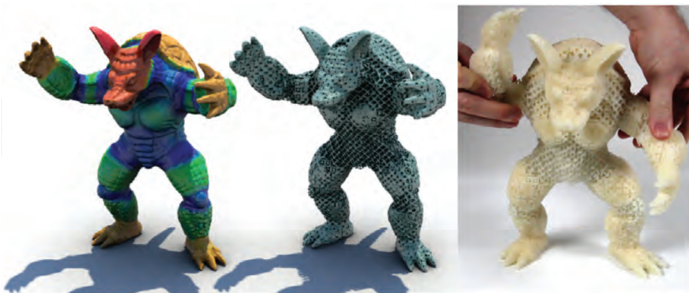
Figure 2.3: Elastic object fabricated with [56]. Color on the leftmost image represents user-specified elasticity parameters. This figure is adapted from the Figure 1 of [56].
