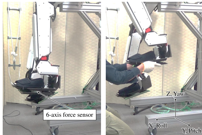
Fig 4.16: Back drivability assessment of the leg part of the exo-skeleton with the attached 6-axis force sensor
