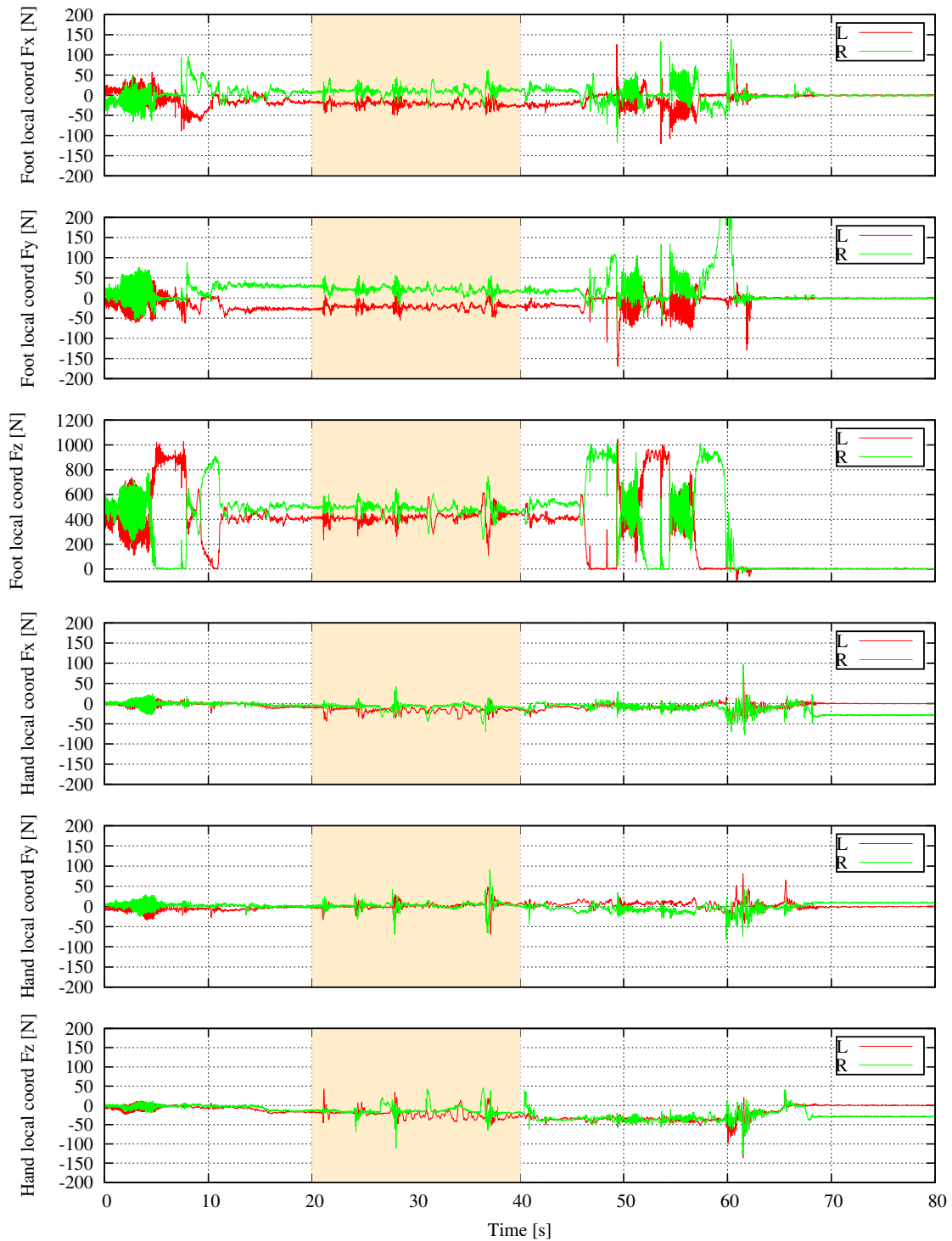
Fig 6.11: End effector force plot of the light weight bilateral dual arm manipulation
