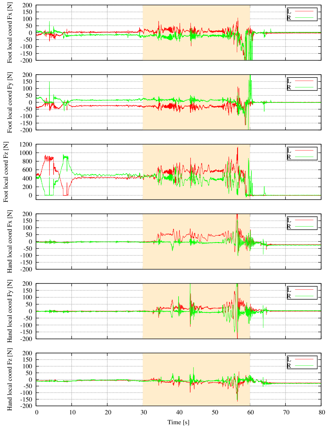
Fig 6.14: End effector force plot of the heavy weight bilateral dual arm manipulation
