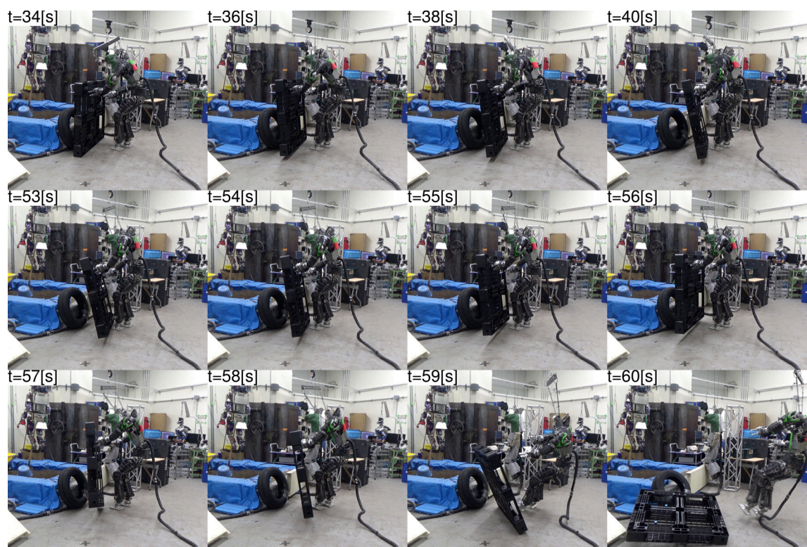
Fig 6.12: Recorded video shots of the heavy weight bilateral dual arm manipulation
