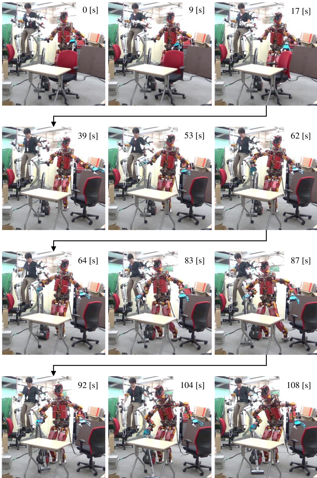
Fig 6.5: Sample house work operation with the whole body bilateral tele-operation system
