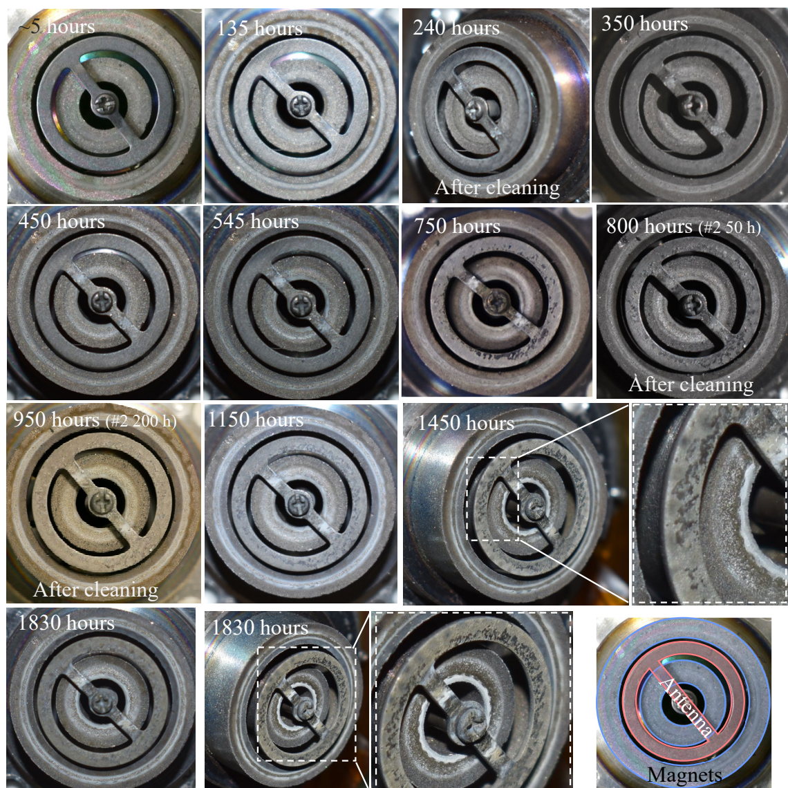
Fig. 4.12 Discharge chamber antenna and magnets contamination of ion thruster long-time operation.
