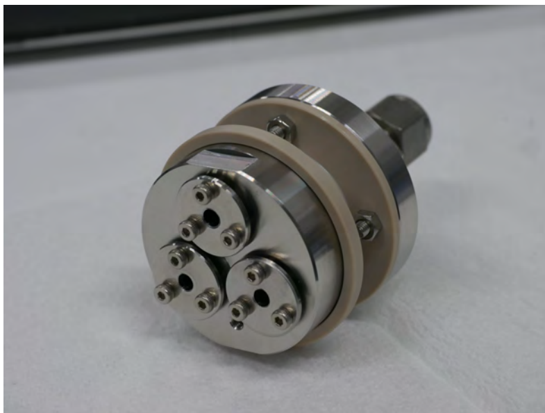
図 2.6: Picture of the gas Isolator.
