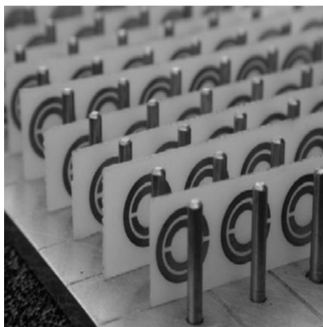
Fig. 1.3 The first example to achieve negative refractive index by using metal strip and split ring resonator[17].
