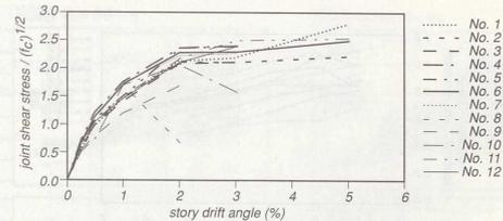
Fig. 8 : Relation of story shear and joint shear evaluated with Eq. (1) at peaks load<sup>8)</sup>
