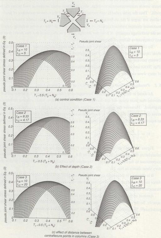
Fig. 21 : Example solution for pseudo joint shear calculated by the new model
