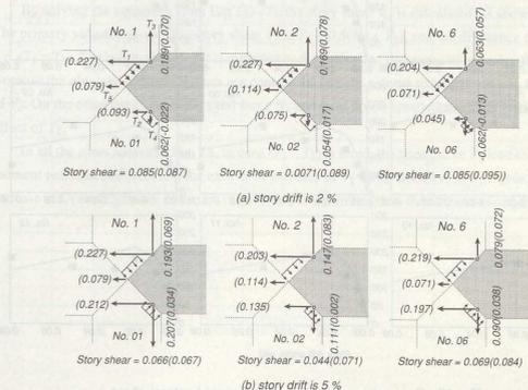
Fig. 18: Predicted column shear by the model (number in parentheses is observed value)
