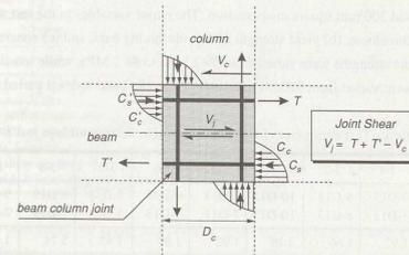
Fig. 1 : Definition of horizontal joint shear in R/C beam column joint
