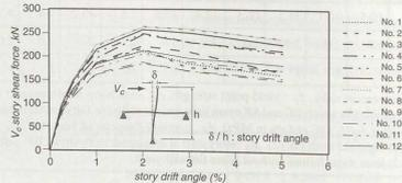
Fig. 3 : Relation of story shear to story drift8)
