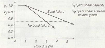
Fig. 9 : Model for joint shear degradation proposed by Priestley<sup>9)</sup>
