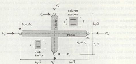
Fig. 17: Geometry of beam-column joint and external forces
