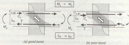
Fig. 11 : Effect of poor bond on moment resistance of beam column joint
