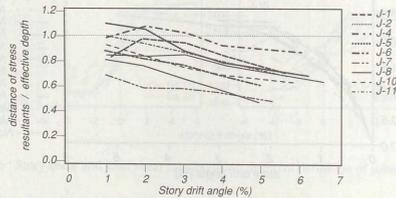
Fig. 10 : Change of the length  $l_{jb}$  (moment lever arm length) at the column face calculated from observed moment and stress in tensile reinforcing steel
