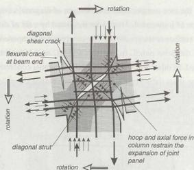
Fig. 14: Joint failure mechanics and force flow among adjacent members
