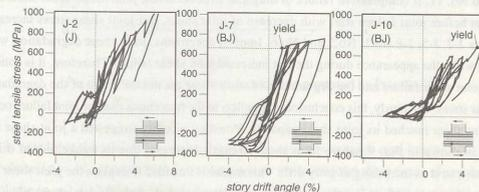
Fig. 5 : Typical relation of story drift and tensile stress in first outer tensile reinforcement
