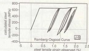
Fig. 4 : Example of stress-strain relation predicted using Ramberg-Osgood model
