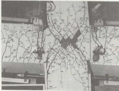
Photo 1 : Observed crack pattern after test (specimen J-7)
