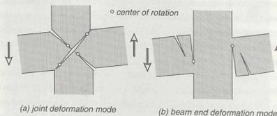
Fig. 15: Joint failure mechanics model
