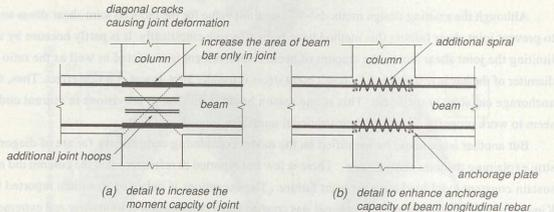
Fig. 22: Probable reinforcing detail to prevent joint shear failure
