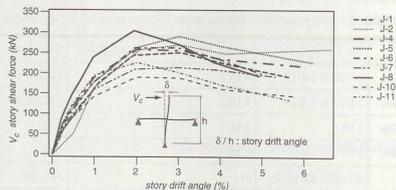
Fig. 2 : Relation of story shear to story drift7)
