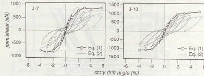
Fig. 6 : Story shear and joint shear relation using different definition of joint shear
