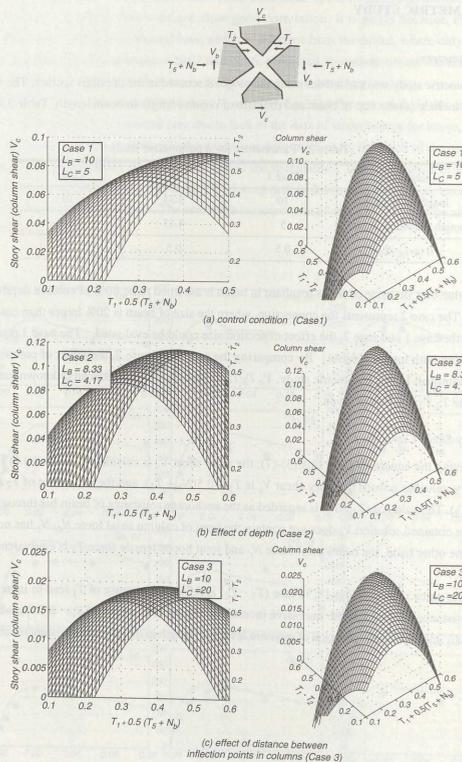
Fig. 20 : Example solution for story shear  $V_c$  calculated by the new model
