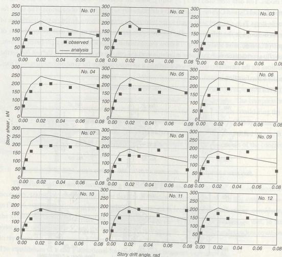
Fig. 19: Comparison of analysis and observed column shear
