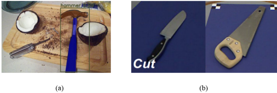
Fig. 2.2: Image based affordance datasets: (a) IIT-AFF [2]: object parts that afford different actions are annotated with different colors. Actions and object functions are regraded as affordance in this dataset. (b)RGB-D Part Affordance Dataset [3] contains RGB-D images and ground-truth affordance labels for 105 kitchens, workshop, and garden tools, and 3 cluttered scenes. Different concepts such as "cut" and "scoop" are all used as affordance.
