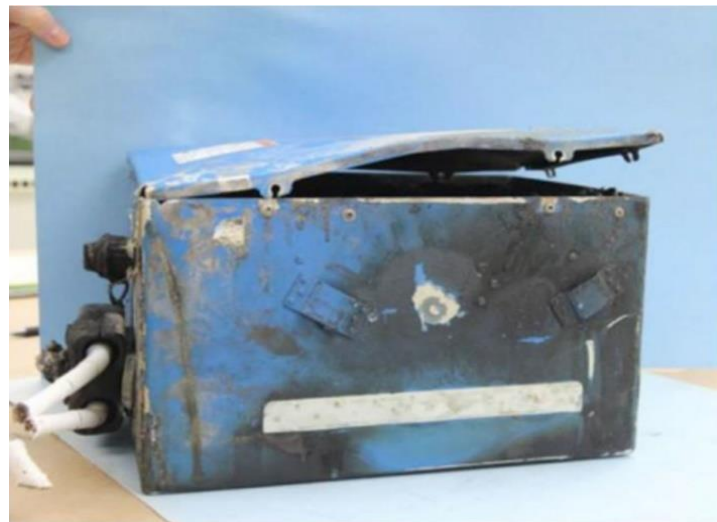
Figure 1.2 Evident damage in the battery after runaway.[11]
