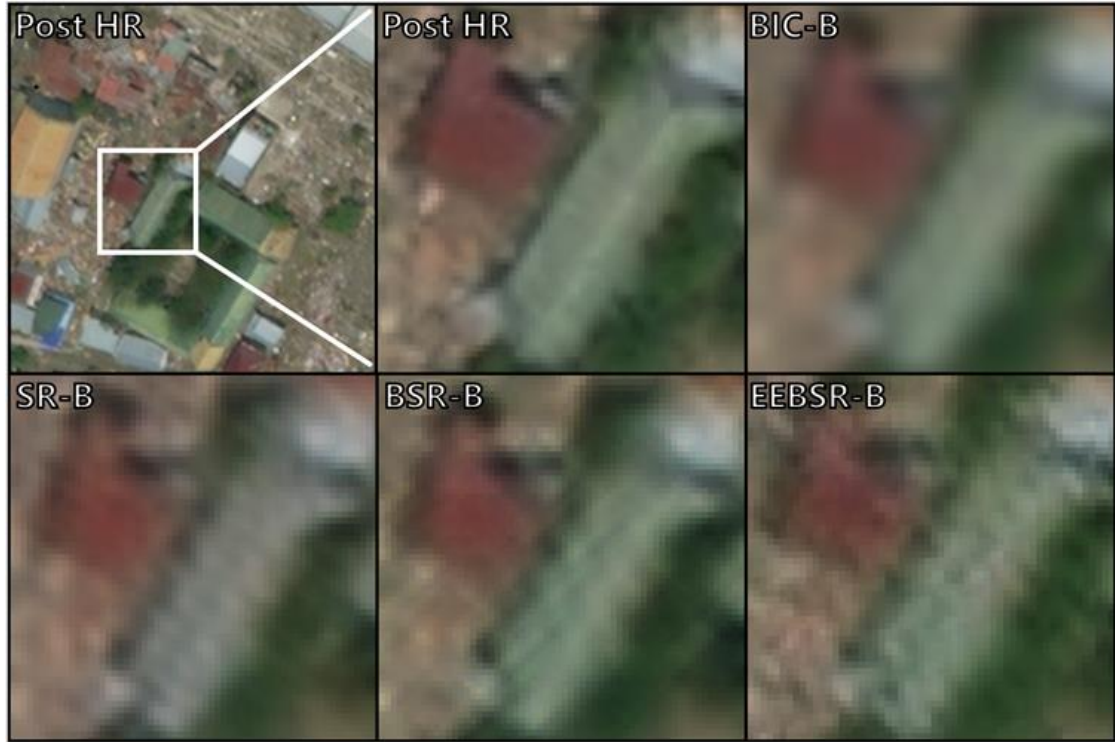
Figure 4.5 The upsampling result in the BIC-B framework and the output of the SR module of the SR-B, BSR-B and EEBSR-B frameworks (zoomed in, LR = 1/4)
