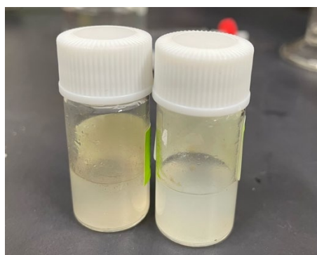
Figure 3-4 Liquid samples pictures, 480°C, 2wt%, 15min (left), 30min (right)
