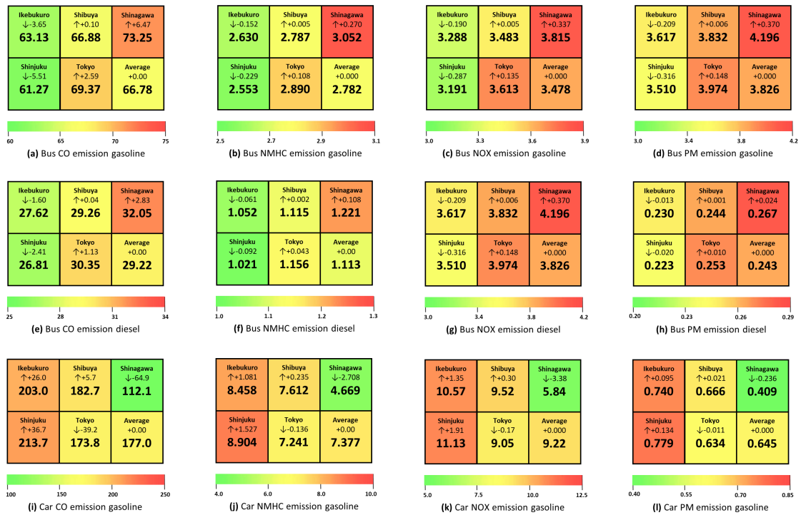
Fig.4.8: (a)average MaaS bus CO emission in grams while using gasoline, (b)average MaaS bus NMHC emission in grams while using gasoline, (c)average MaaS bus NOX emission in grams while using gasoline (d)average MaaS bus PM emission in grams while using gasoline, (e)average MaaS bus CO emission in grams while using diesel, (f)average MaaS bus NMHC emission in grams while using diesel, (g)average MaaS bus NOX emission in grams while using diesel, (h)average MaaS bus PM emission in grams while using diesel,(i)average car CO emission in grams while using gasoline, (j)average car NMHC emission in grams while using gasoline, (k)average car NOX emission in grams while using gasoline, (l)average car PM emission in grams while using gasoline
