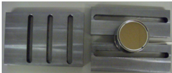
Figure 5.8: The lead collimator used in 2008. The thickness is 1.8 cm, width of the slit is 1 cm, and a 2-inch PMT is superimposed as a reference.
