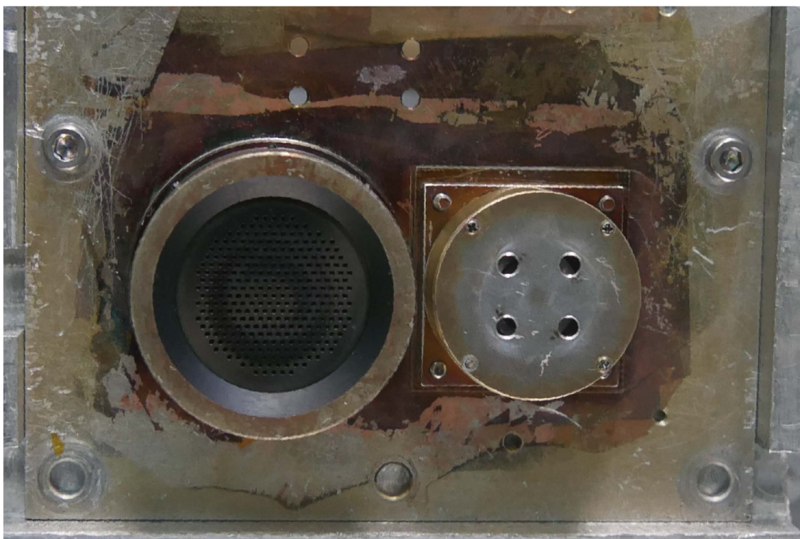
Figure 3-4 Ion thruster: Ion source (left) and neutralizer (right)
