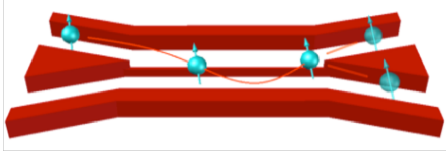
Figure 3.1: Electron-tunneling process in a tunnel-coupled wire.
