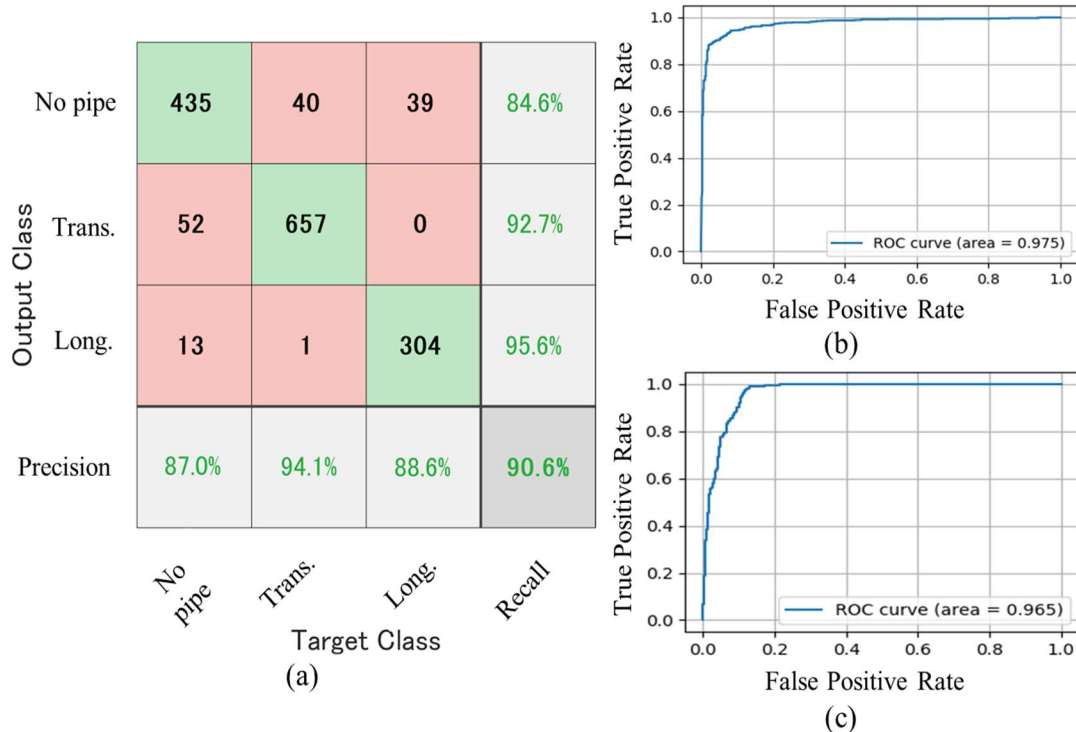
Fig. 6.52 Three-category classification of transverse and longitudinal pipes (a) confusion matrix (b) transverse pipe ROC (c) longitudinal pipe ROC
