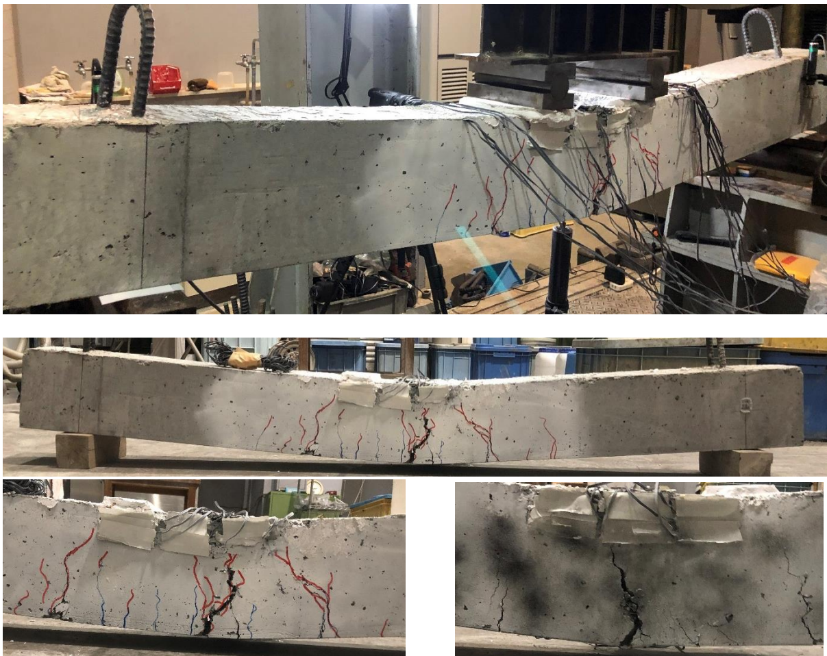
Fig. 4.15 Beam FBS_01 after failure under static loading.
