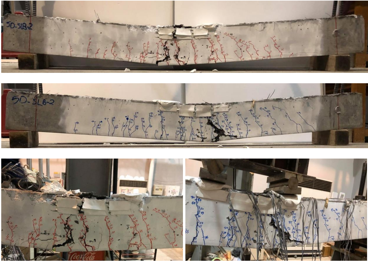
Fig. 7.14 Beam 5D_FBS_02 after failure under static loading.
