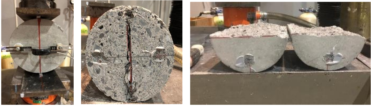
Fig. 4.9 Splitting tensile test.
