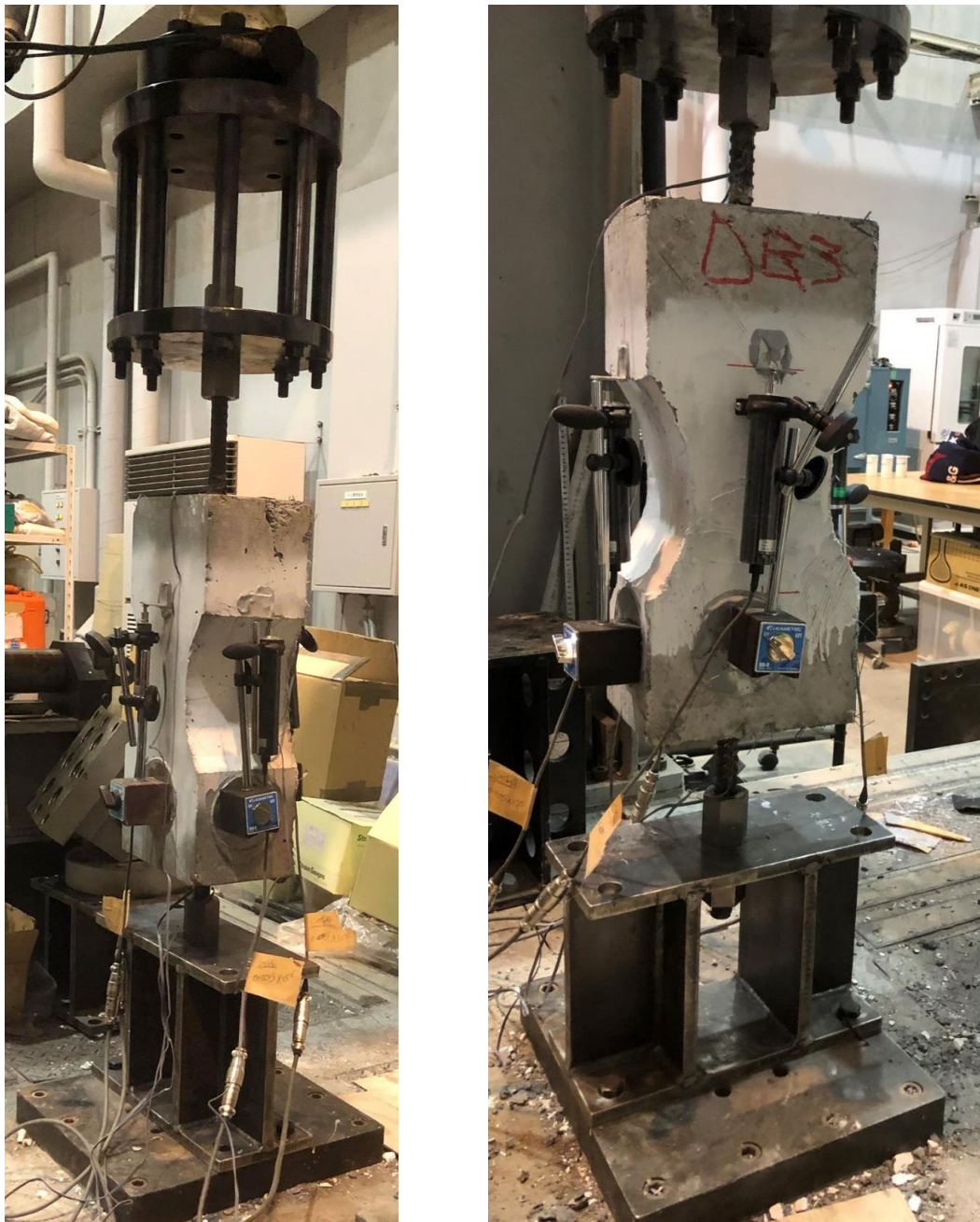
Fig. 7.4 The dog-bone SFRC specimens with the attached transducers.
