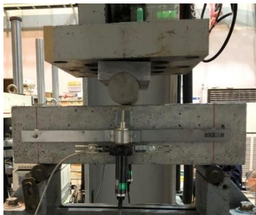
Fig. 4.10 Bending test on prismatic SFRC specimens.
