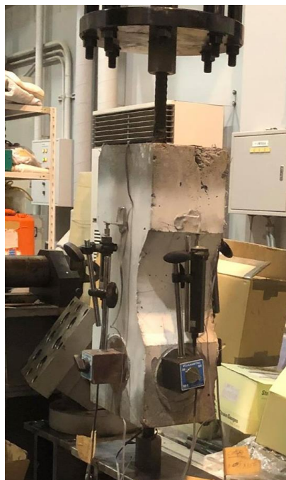
Fig. 3.9 Dog-bone uniaxial tensile test.
