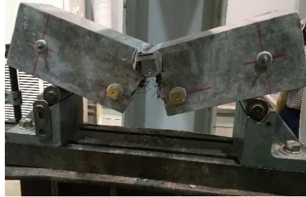
Fig. 4.12 Fracture of SFRC prismatic specimen at the end of the bending test.
