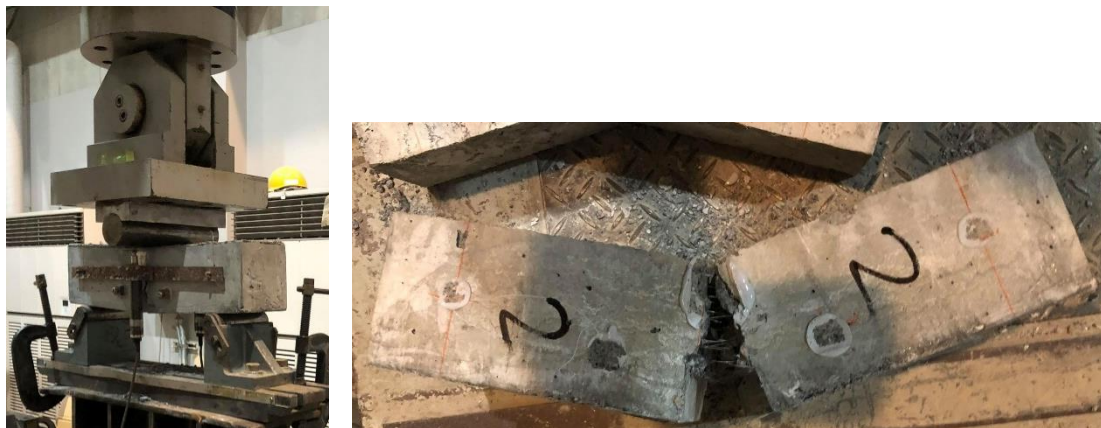
Fig. 6.1 Fracture of SFRC prismatic specimen at the end of the bending test.
