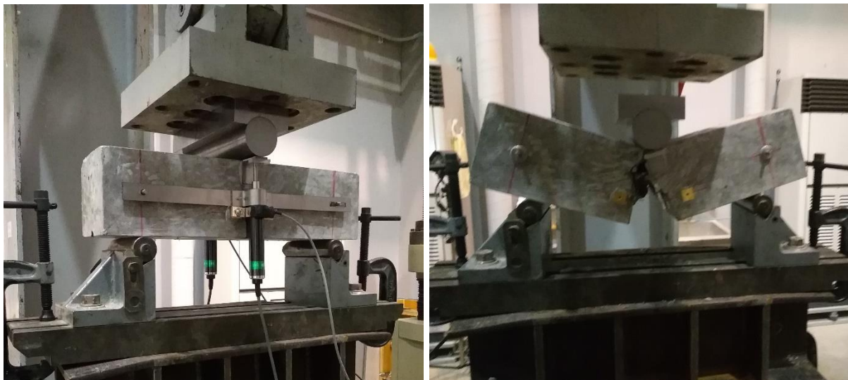
Fig. 5.3 Fracture of SFRC prismatic specimen at the end of the bending test.
