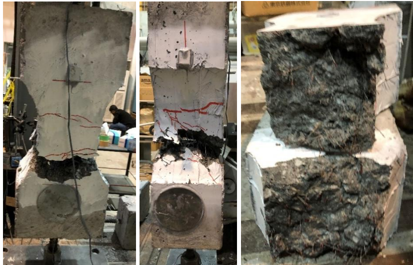
(b) The rupture of specimen DB_02.
