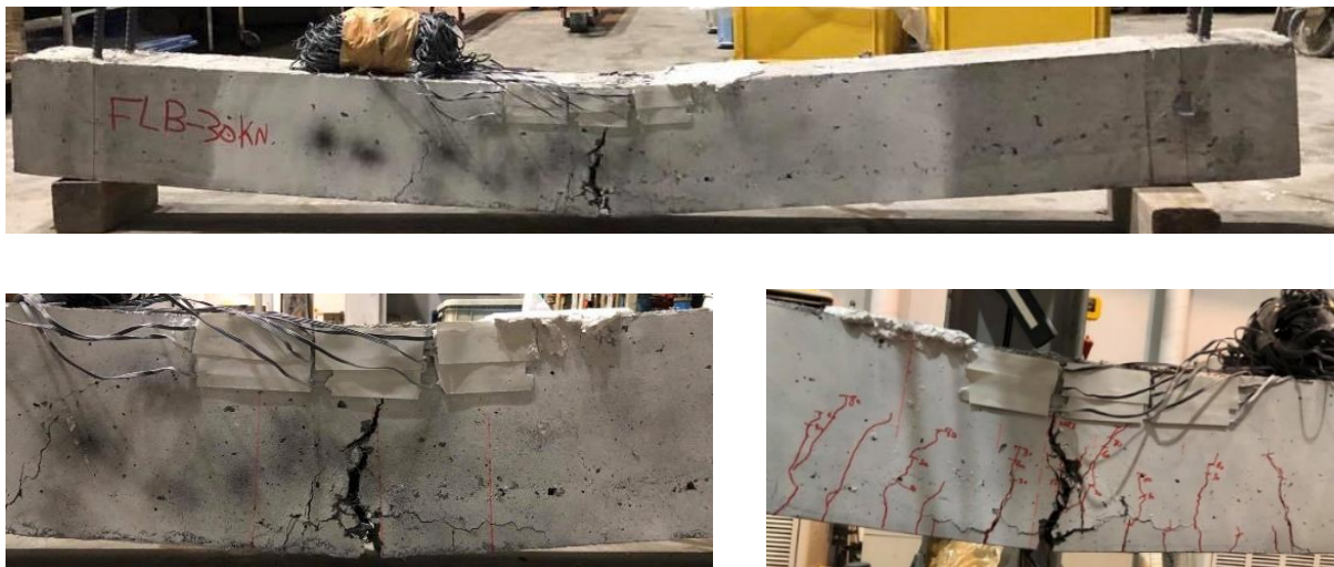
Fig. 4.19 Beam FBF_30 over fatigue life under flexural cyclic loading.
