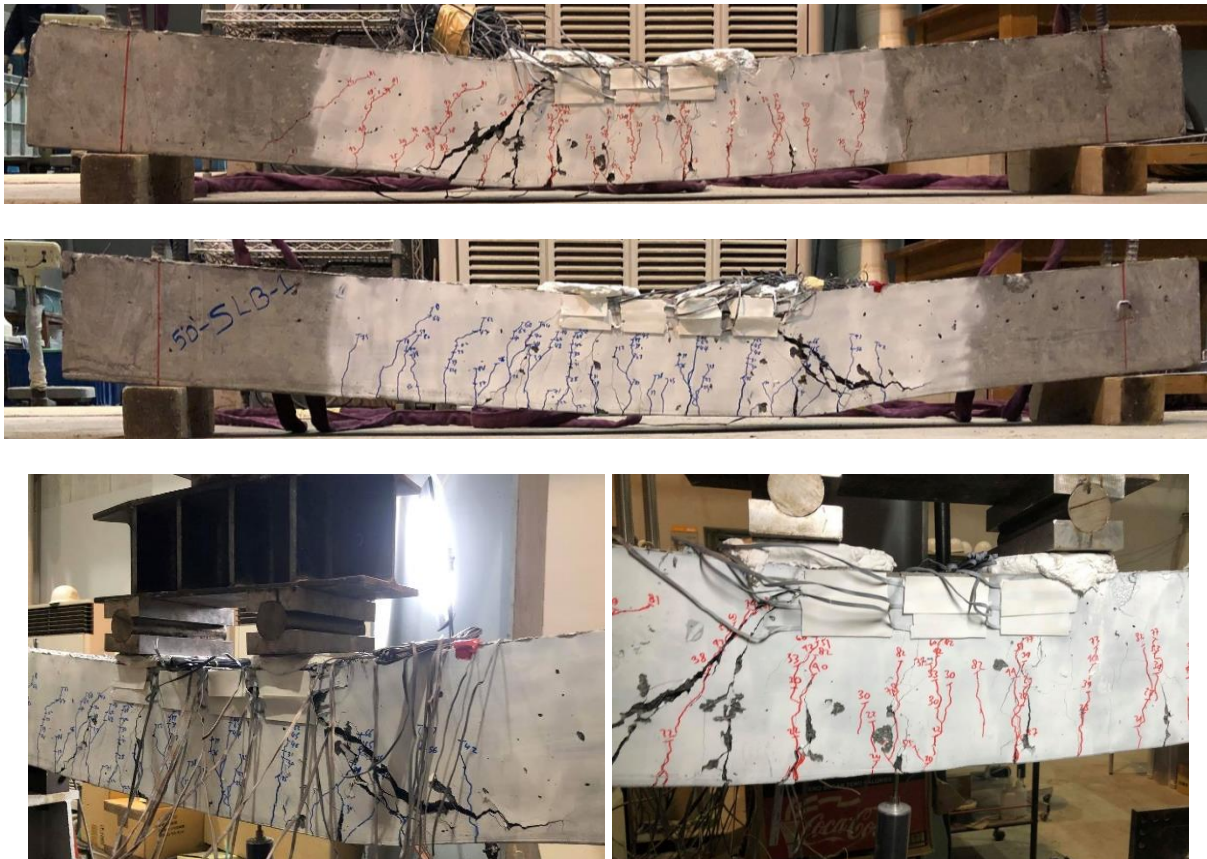
Fig. 7.9 Beam 5D_FBS_01 after failure under static loading.
