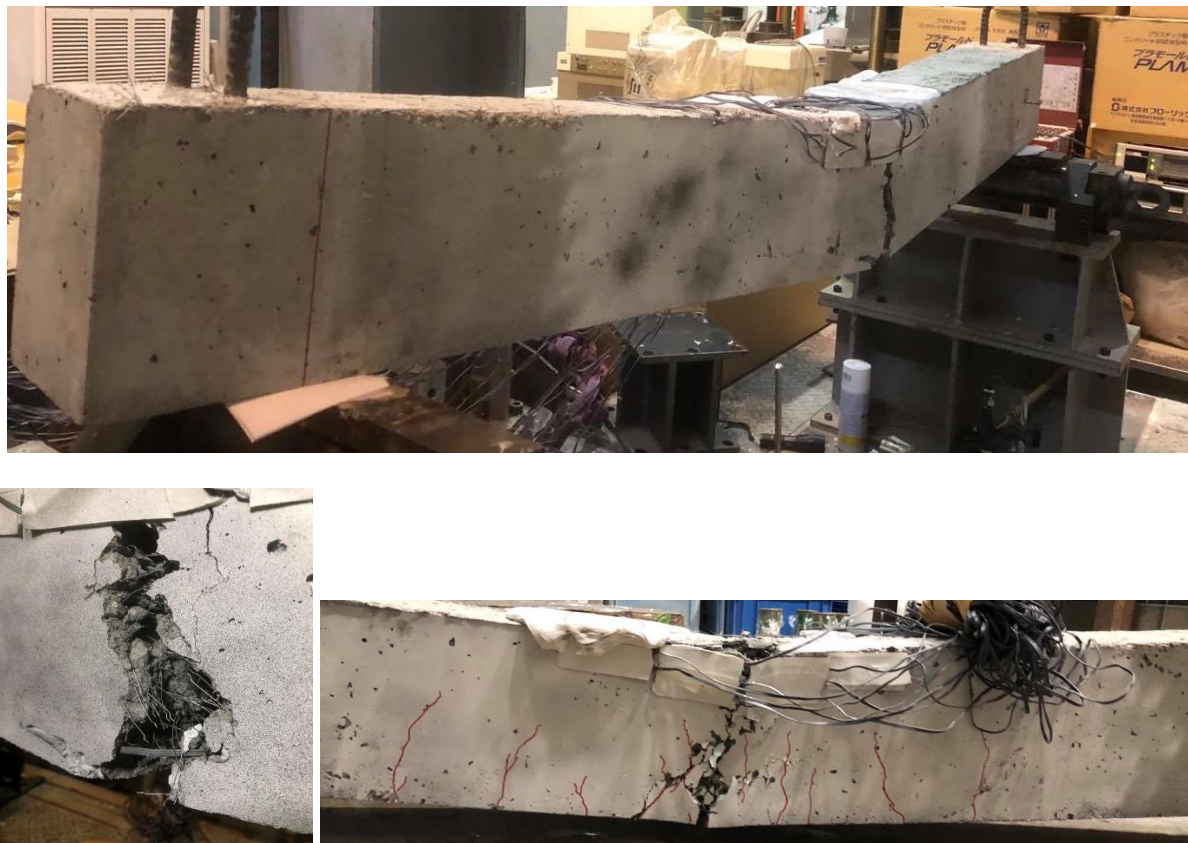
Fig. 4.31 Beam FBF_50 over fatigue life under flexural cyclic loading.
