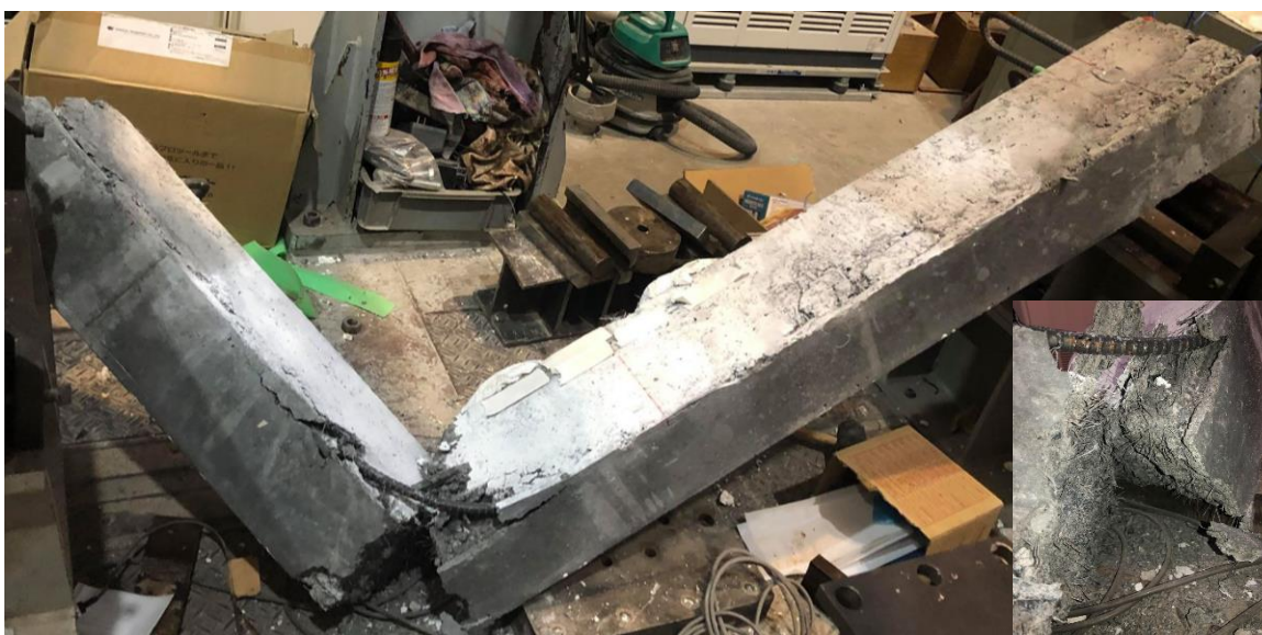
Fig. 6.46 Beam D13_FBF_40 over fatigue life under flexural cyclic loading.
