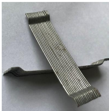
Fig. 4.2 Hooked-end steel fibers.
