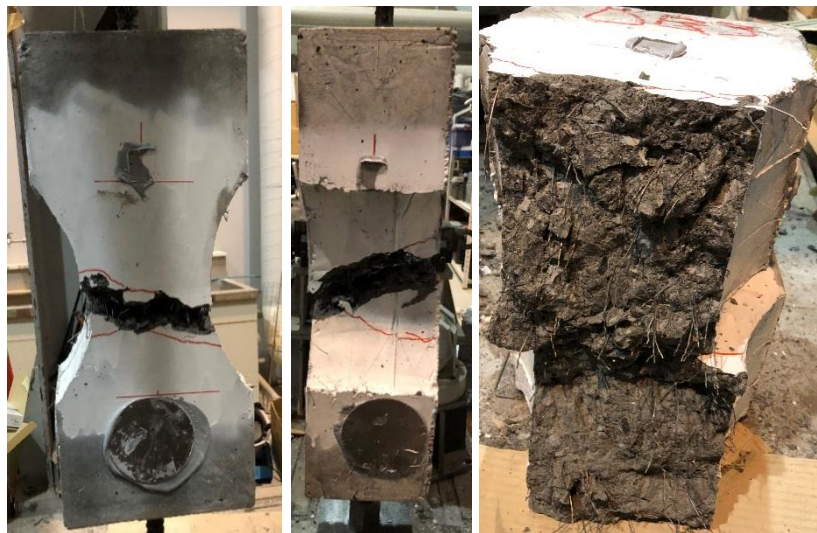
(c) The rupture of specimen DB_03.
