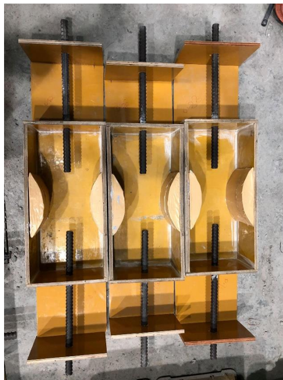
Fig. 7.2 Formwork of the dog-bone SFRC specimen.
