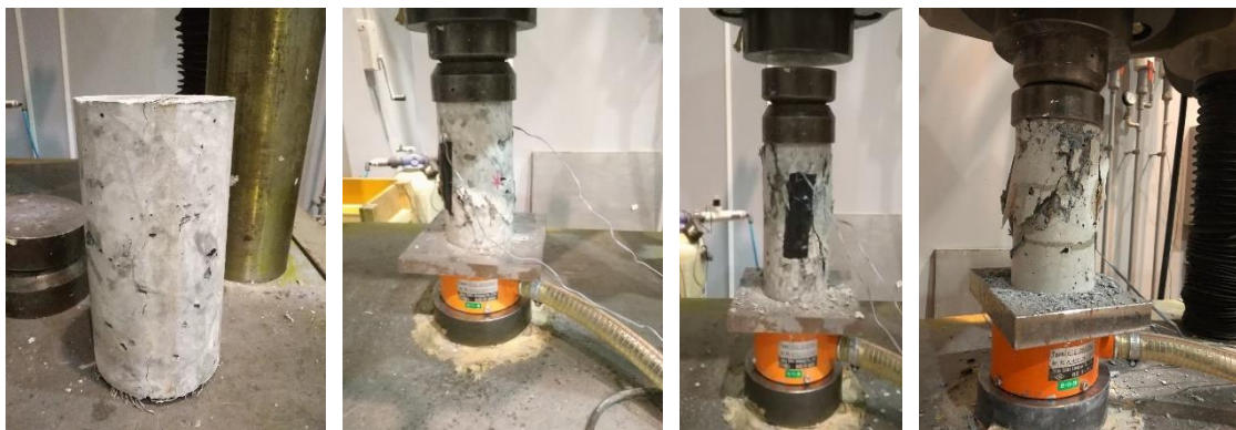
Fig. 4.8 Concrete compressive test.
