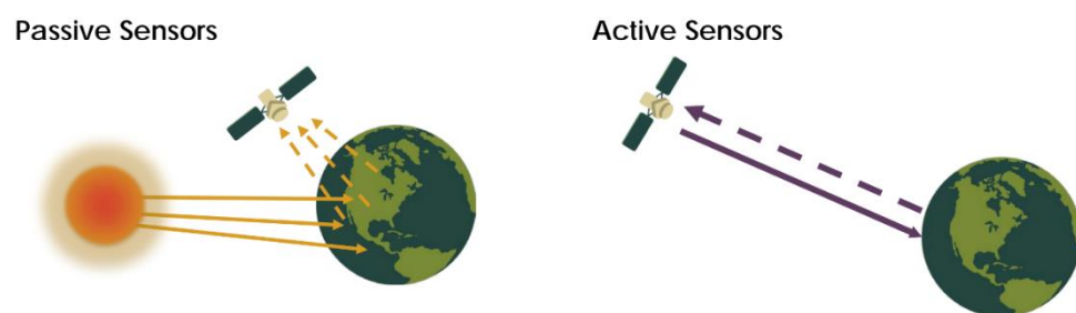
Figure 2.5. Two types of sensors used in remote sensing (RS) (NASA).
