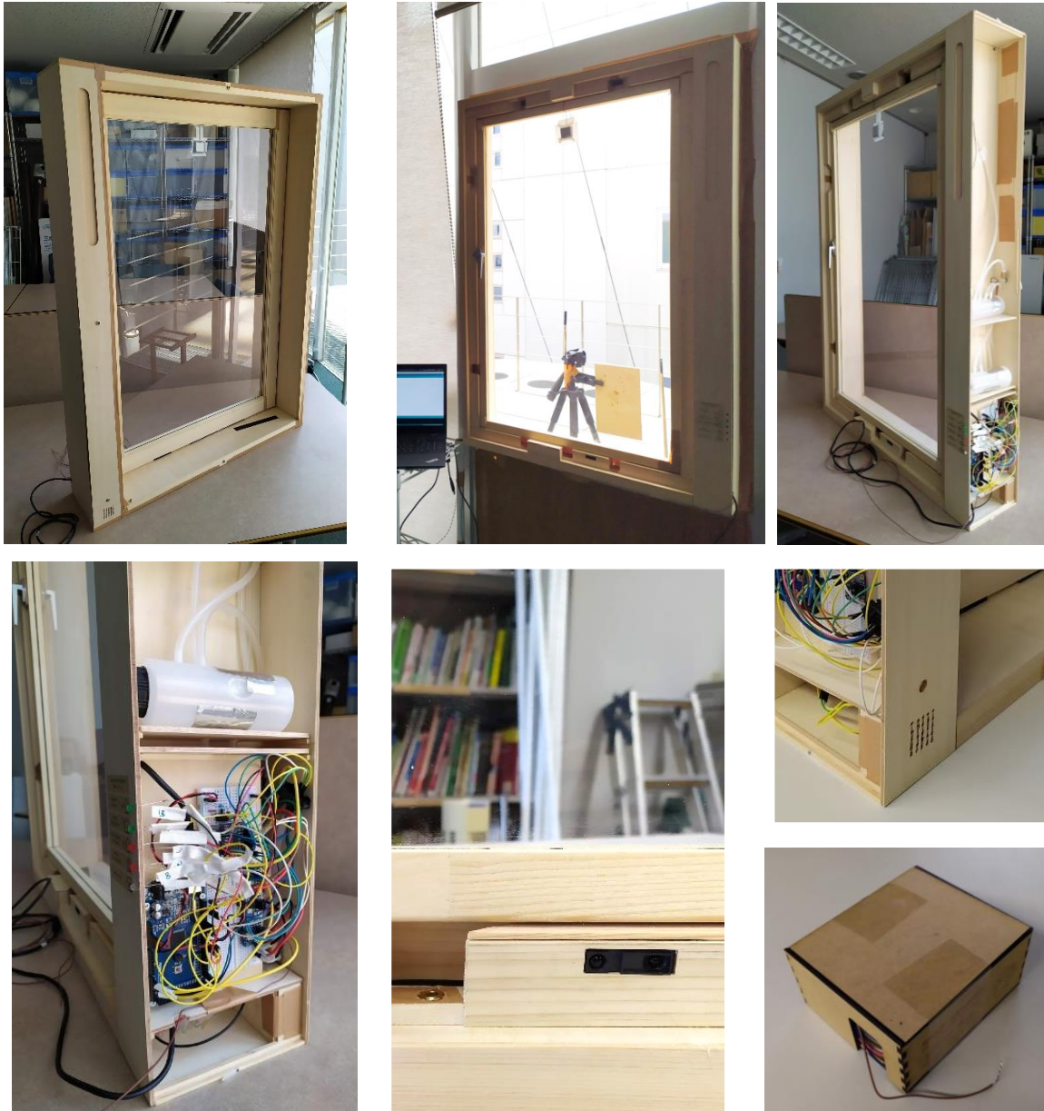
Figure 74. The main window prototype (above), details (below left and center), and the image of the wall device (below right).
