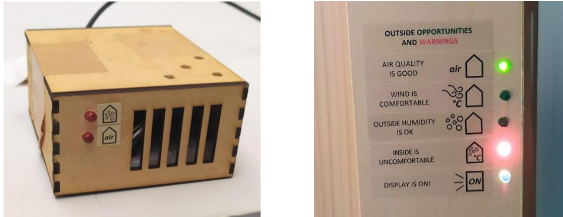
Figure 85. Pictures of the comfort/discomfort LEDs inserted in the wall device (left), and on the internal sash of the main window (right). A white led was added to simulate when the display was on.
