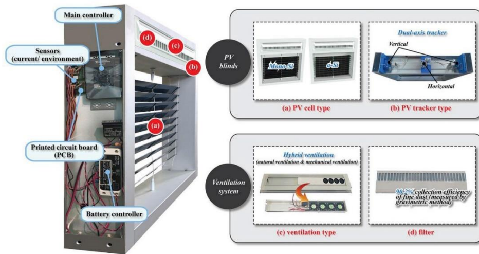
Figure 13. A prototype of a multi-function smart window for ZEB buildings. From W Jung, et al. (2019).
