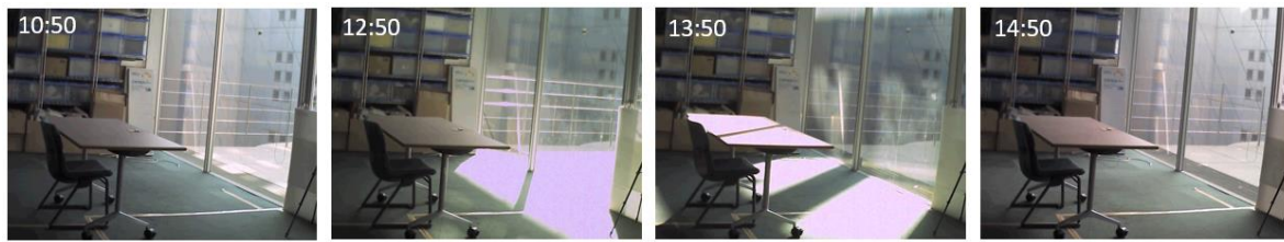
Figure 24. Time sequence illustrating solar radiation inside the meeting room with open curtains.
