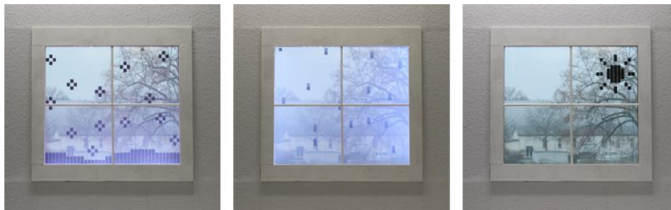
Figure 12. Weather information displayed by the WindowWall system. From Bader et al. (2019).
