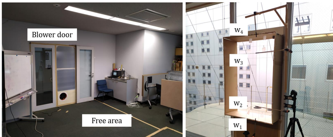
Figure 68. Testing room with the blower door (left), and the special cardboard device with the anemometers in position (right).
