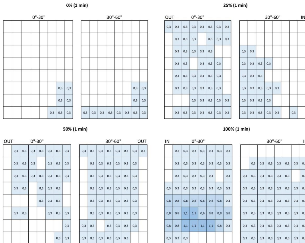
Figure 66. Example proceeding from the video analysis of the window mesh. The image shows the 15:00 session with 1- minute patterns depending on the opening percentage of the opposite door. In particular (IN) is ingoing, and (OUT) is outgoing wind.
