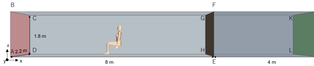
Figure 4-4. Simulation model of the wind tunnel.
