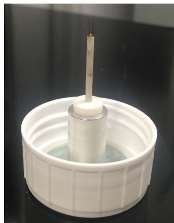
Figure 3-13. Miniature wire probe (55P11) produced by Dantec Dynamics.
