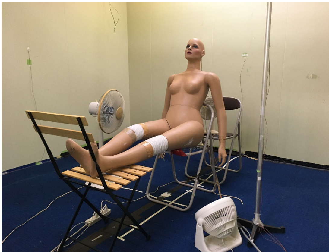
Figure 3-3. Thermal manikin during calibration.
