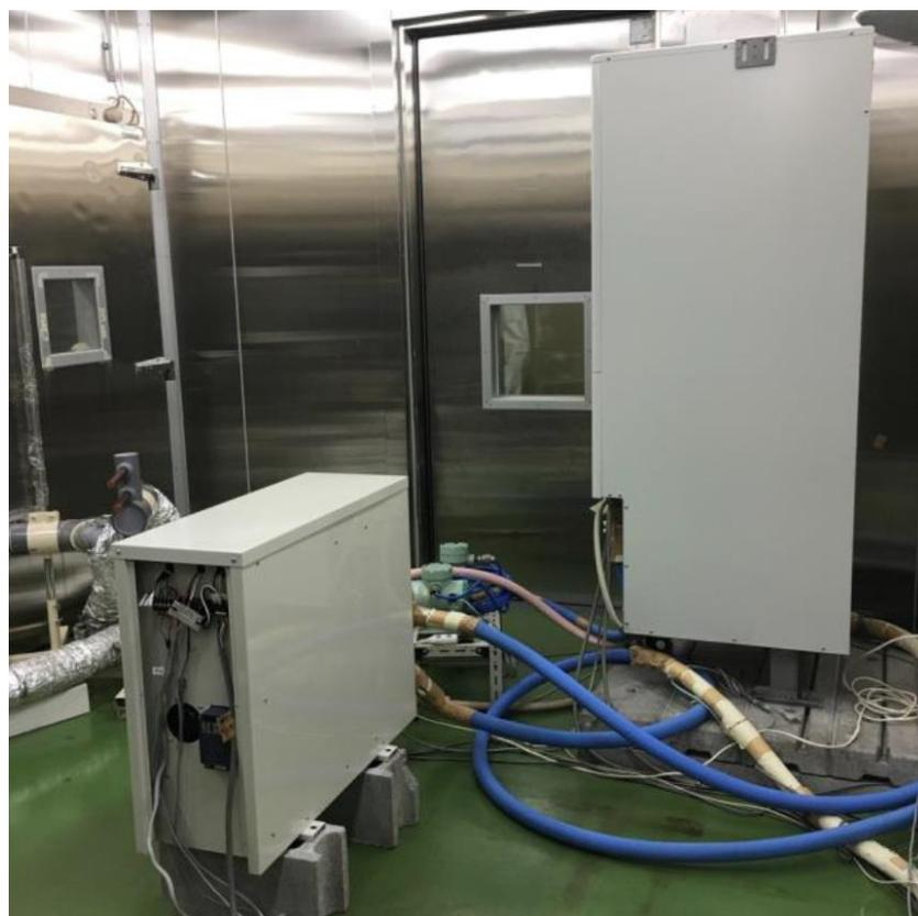
Figure 3. 41 Performance test of hot water supply heat pump in cold weather(test room).
