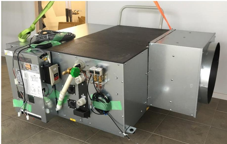
Figure 3. 36 Appearance of the prototype water source heat pump for air conditioning.
