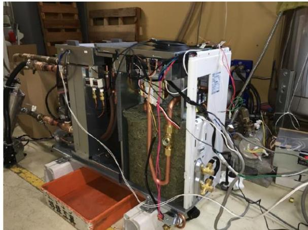
Figure 3. 29 Performance test of a prototype heat pump for floor heating
