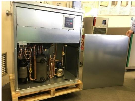
Figure 3. 11 Compressor unit of sky source heat pump.
