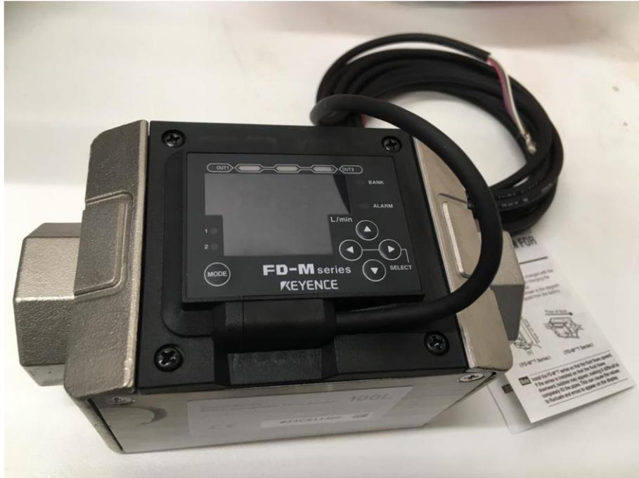
Figure 4. 13 flow meter for measuring the flow rate of circulating water.
