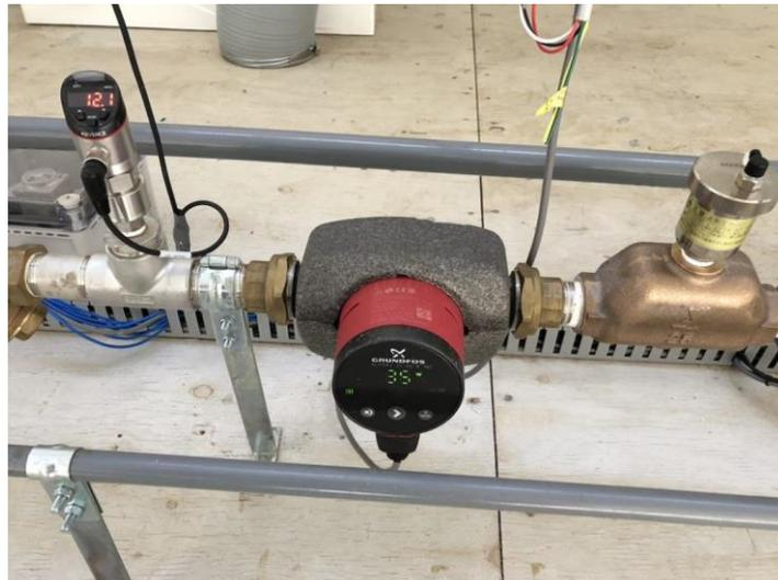
Figure 3. 4 Small DC water pump (Grundfos ALPHA2)
