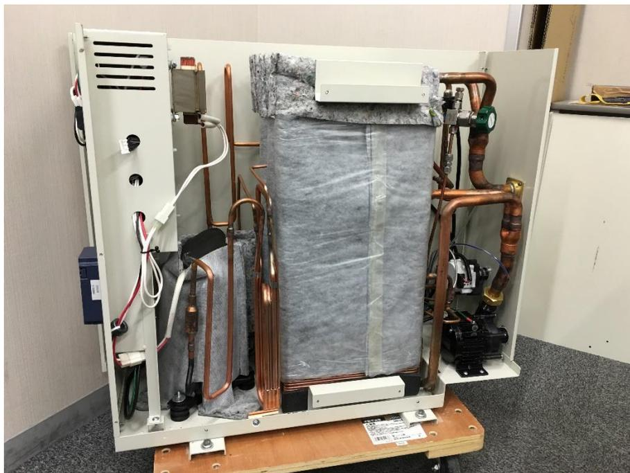
Figure 3. 40 Structure of water source heat pump for domestic hot water supply prototype.
