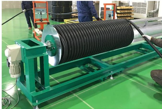
Figure 3. 27 Manufacture of double-helical ground heat exchanger
