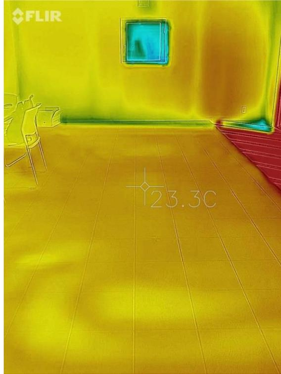
Figure 3. 33 Infrared photography of floor heating. (when circulating hot water is 28 °C)
