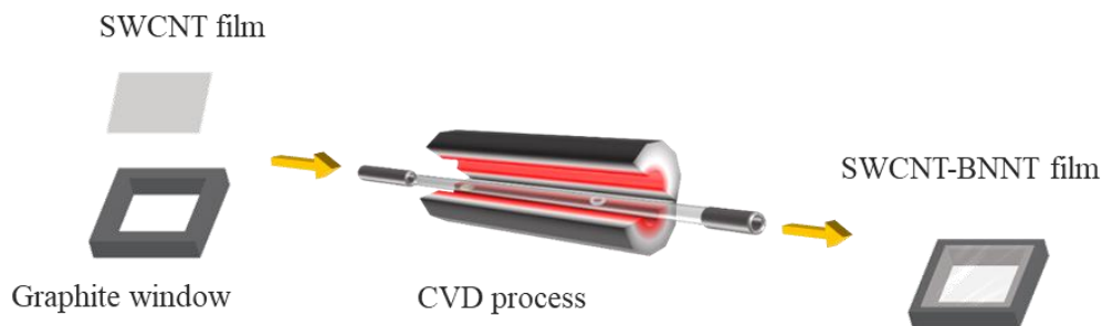
FIG 4-2. Schematic of the CVD process for BNNT growth on an SWCNT template suspended on graphite window.
