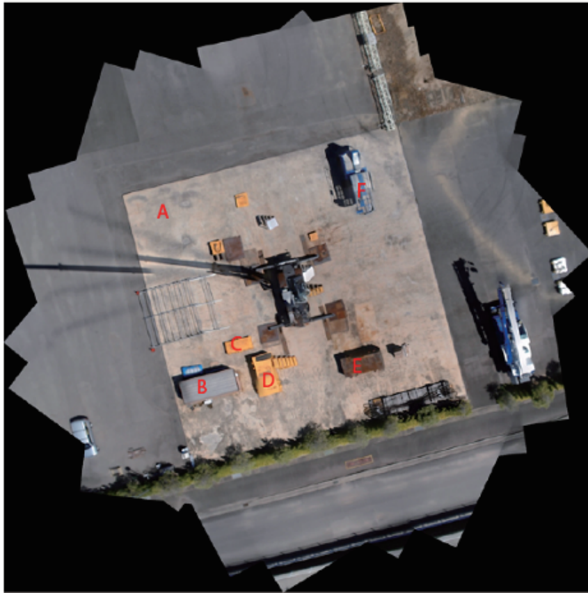
Fig. 4.9: Features and objects which are used to verify the workspace map's metric property.
