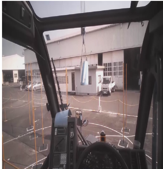
Fig. 1.2: The operation cabin of a rough crane
