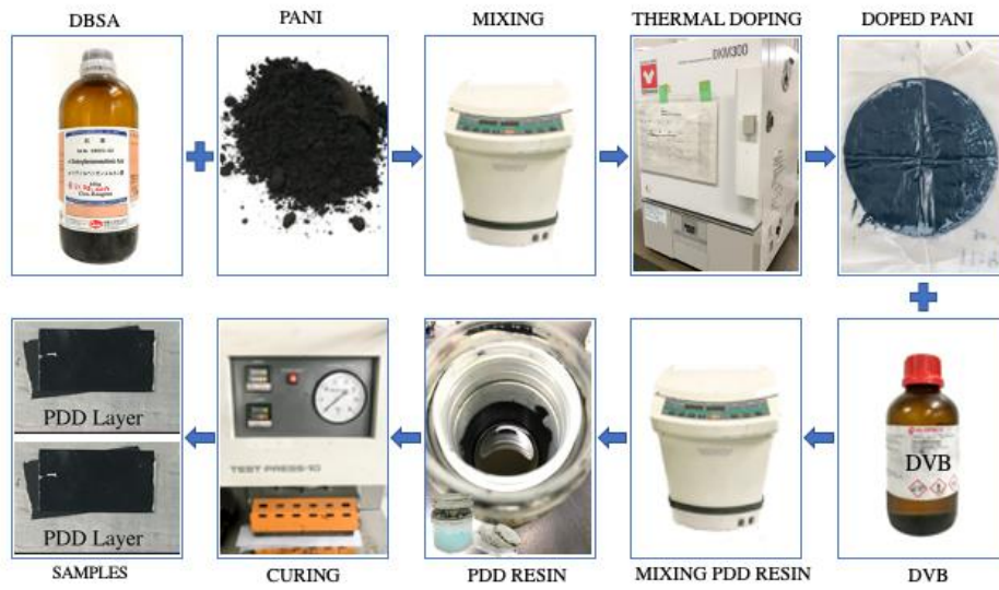
Figure 11: Fabrication process of polyaniline based novel polyaniline-based conductive polymer system.
