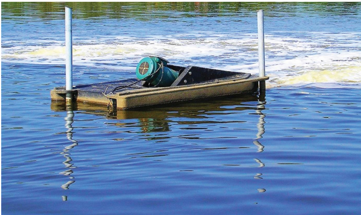
Figure 2.2 Propeller-aspirator pump [19].
