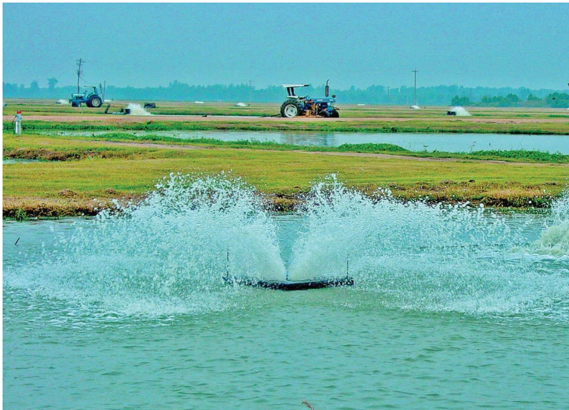
Figure 2.3 Vertical pump sprayer [19].
