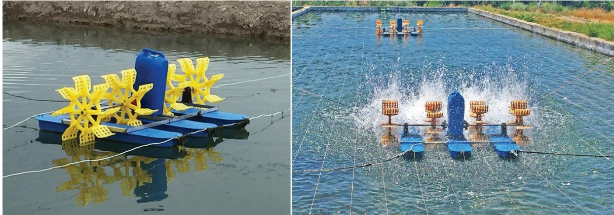
Figure 2.4 Paddlewheel aerators [19].
