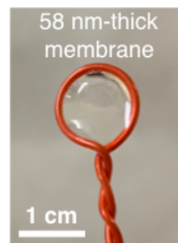
Figure 1. Photograph of a free-standing 58-nm thick artificial lignin membrane transferred to a wire lasso, together with its proposed chemical structure.
