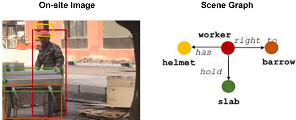
Figure 2.6: An example of the scene graph-based approach for hazard identification.
