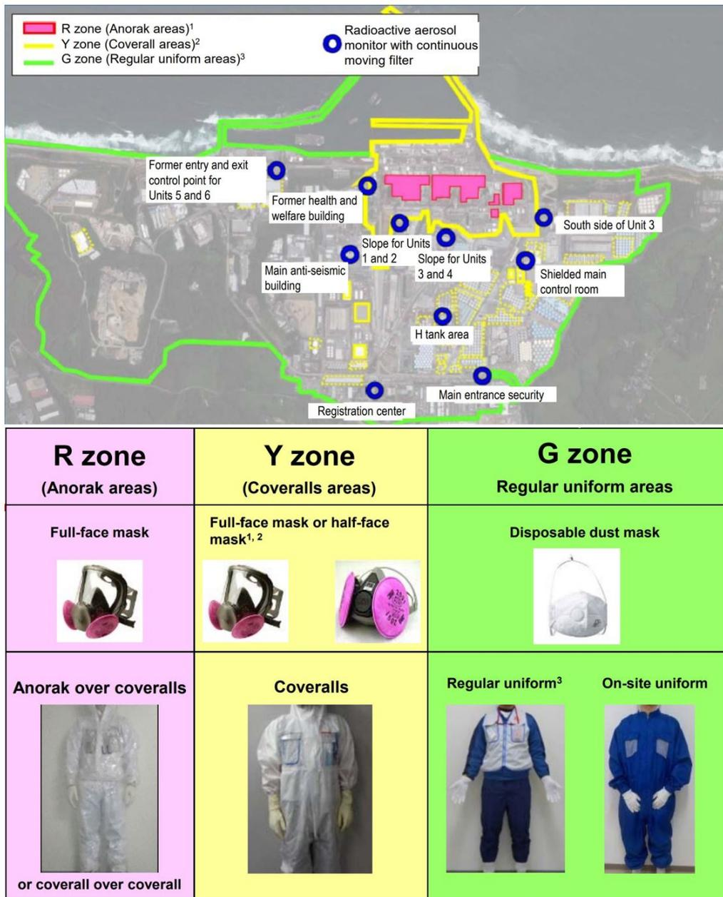
Figure 1.2: PPE requirements for each zone in Fukushima Daiichi NPS.
