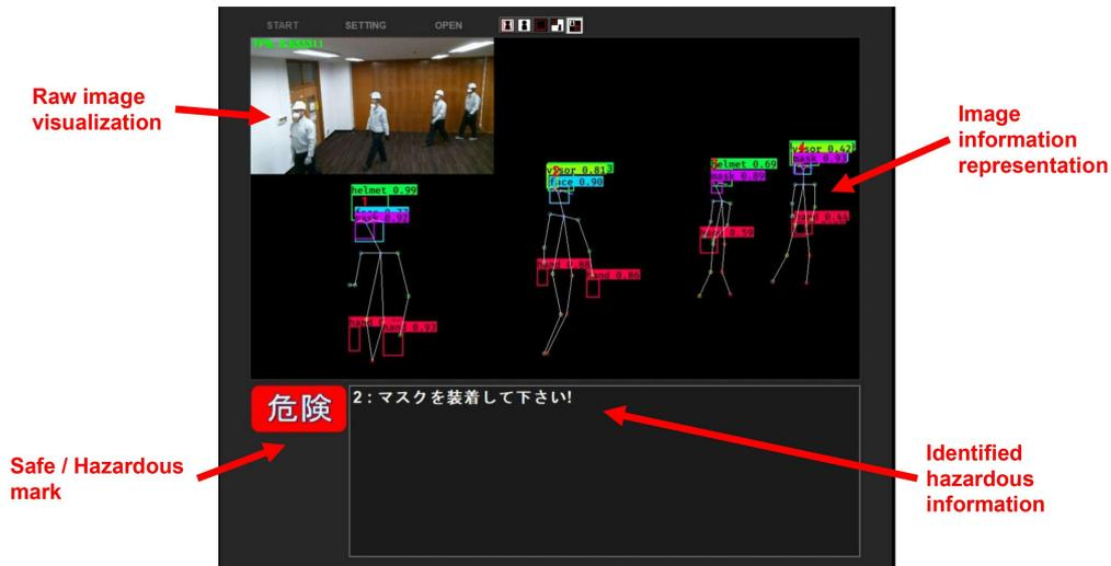
Figure 5.3: UI of the real-time on-site hazards identification system.
