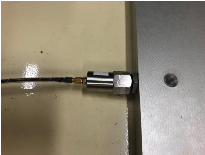
Figure 2-7 One accelerometer used in experiments
