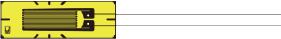
Figure 2-8 Strain gauge used in experiments
