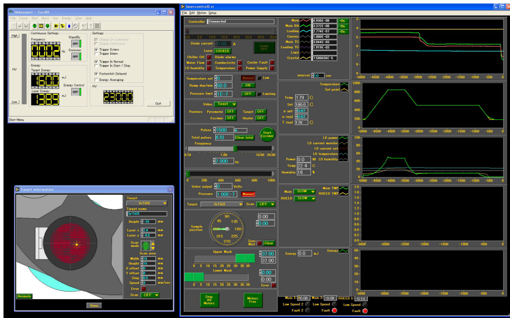
Figure 3.5: LabVIEW control panel for monitoring and controlling the PLD process parameters.
