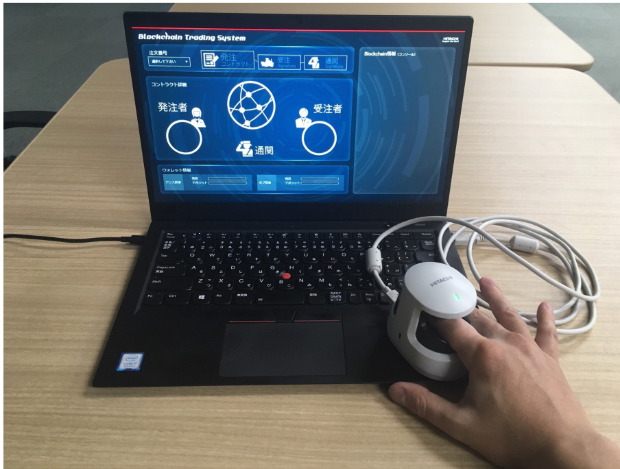
Figure 4.4: Implementation of biometrics-based fuzzy signature on Hyperledger Fabric
