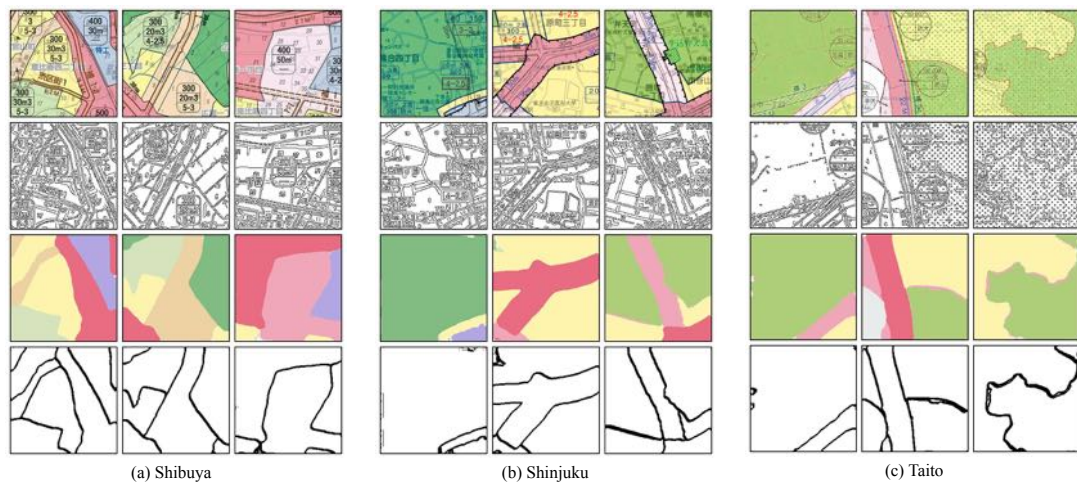
FIGURE B.9: Map denoising and outline extraction. First row: the original scanned map; second row: canny edge detection results of the original scanned map; third row: denoised map; fourth line: extracted outline for different region.
