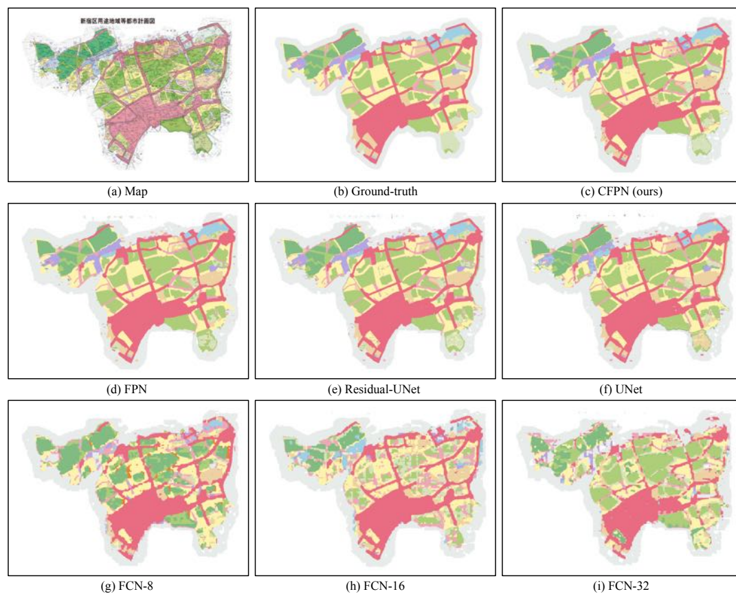
FIGURE B.3: Segmentation results obtained by different methods for urban planning map of Shinjuku district.
